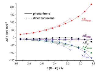
Fig. 3 Comparative energy decomposition analyses for the Diels–Alder cycloaddition reactions involving maleic anhydride and phenanthrene (solid lines) and dibenzoovalene (dashed lines) along the reaction coordinate projected onto the forming C···C bond. All data were computed at the BP86-D3/TZ2P//RI-BP86-D3/def2-SVP level.
