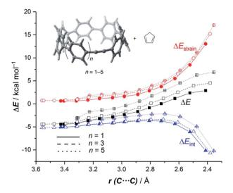
Fig. 9 Comparative activation strain diagrams for the Diels–Alder cycloaddition reactions involving cyclopentadiene and CPPs  $\mathbf{18a}$  (n=1, solid lines),  $\mathbf{18c}$  (n=3, dashed lines) and  $\mathbf{18e}$  (n=5, dotted lines) along the reaction coordinate projected onto the forming C···C bond. All data were computed at the BP86-D3/def2-TZVPP//RI-BP86-D3/def2-SVP level.
