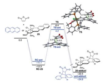
**Fig. 14** Computed reaction profile for the Diels–Alder cycloaddition reaction between maleic anhydride and anthracene (blue lines) and iridaanthracene **25** (black lines). Relative energies and bond distances are given in kcal mol<sup>-1</sup> and angstroms, respectively. All data have been computed at the BP86-D3/def2-TZVPP//RI-BP86-D3/def2-SVP level.
