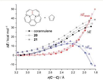
Fig. 11 Comparative activation strain diagrams for the Diels-Alder cycloaddition reactions involving cyclopentadiene and corannulene (solid lines), BN-corannulene 20 (dashed lines) and (BN)2-corannulene 21 (dotted lines) along the reaction coordinate projected onto the forming C···C bond. All data were computed at the M06-2X/def2-TZVPP//M06-2X/def2-SVP level.
