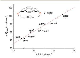
Fig. 8 Plot of the computed activation barriers *versus* the activation strain energies for the Diels–Alder reaction involving pyrenophanes **16** and TCNE. All data were computed at the PCM(benzene)-M06-2X/def2-TZVPP//B3LYP-D3/def2-SVP level.
