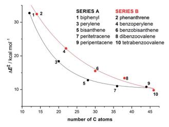
Fig. 1 Plot of the activation barriers *versus* the total number of carbon atoms of planar PAHs **1–10** for the corresponding Diels–Alder reactions with maleic anhydride. Energies were computed at the BP86-D3/def2-TZVPP//RI-BP86-D3/def2-SVP level.
