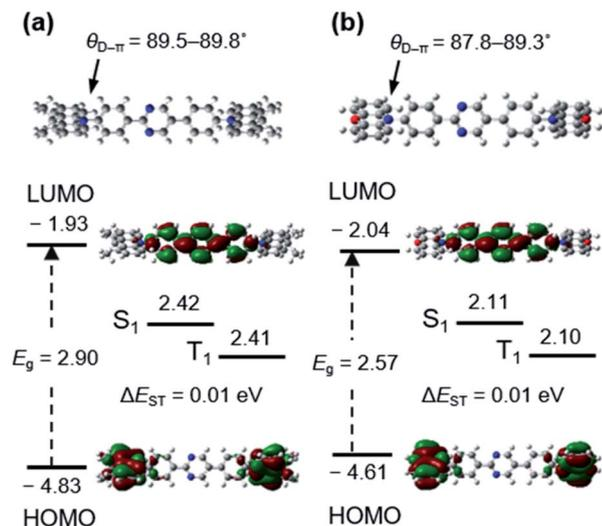
Fig. 1 The optimized molecular structure, singlet ( $S_1$ ) and triplet ( $T_1$ ) energy levels, and HOMO and LUMO distribution of (a) AcPYM and (b) PxBYM calculated via DFT and TD-DFT at the B3LYP/6-31G(d,p) level.
