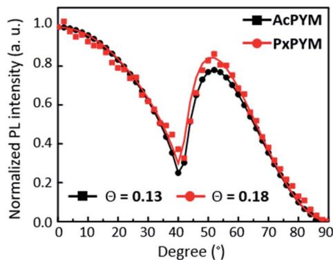
Fig. 4 Angle-dependent PL spectra of AcPYM and PxBYM (*p*-polarized light from 15 nm thin film at 480 nm for AcPYM and 525 nm for PxBYM).  $\theta$  is an anisotropy factor calculated from the fitted solid lines, while the symbols present the experimental data.
