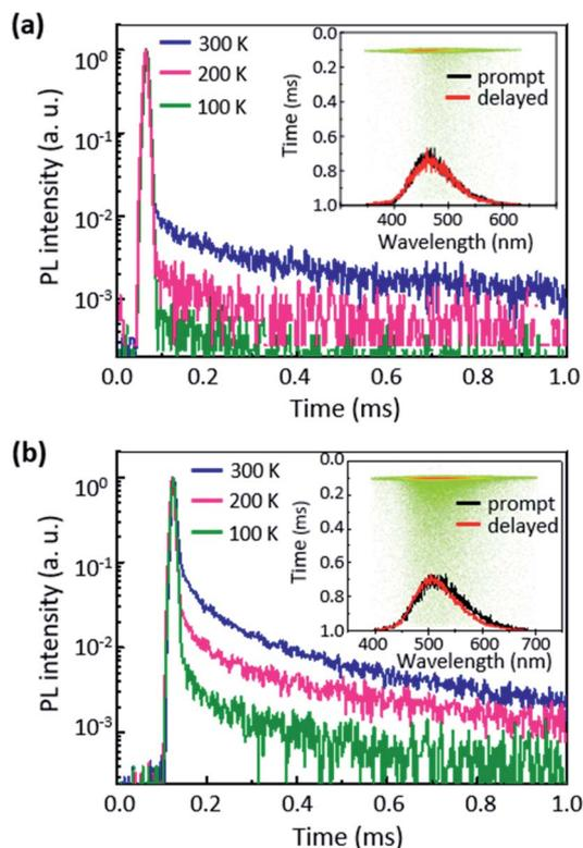
Fig. 3 Transient decay curves of the (a) 6 wt% AcPYM:PPT- and (b) 6 wt% PxBYM:PPT-doped films (inset: time-resolved PL spectra and streak images).
