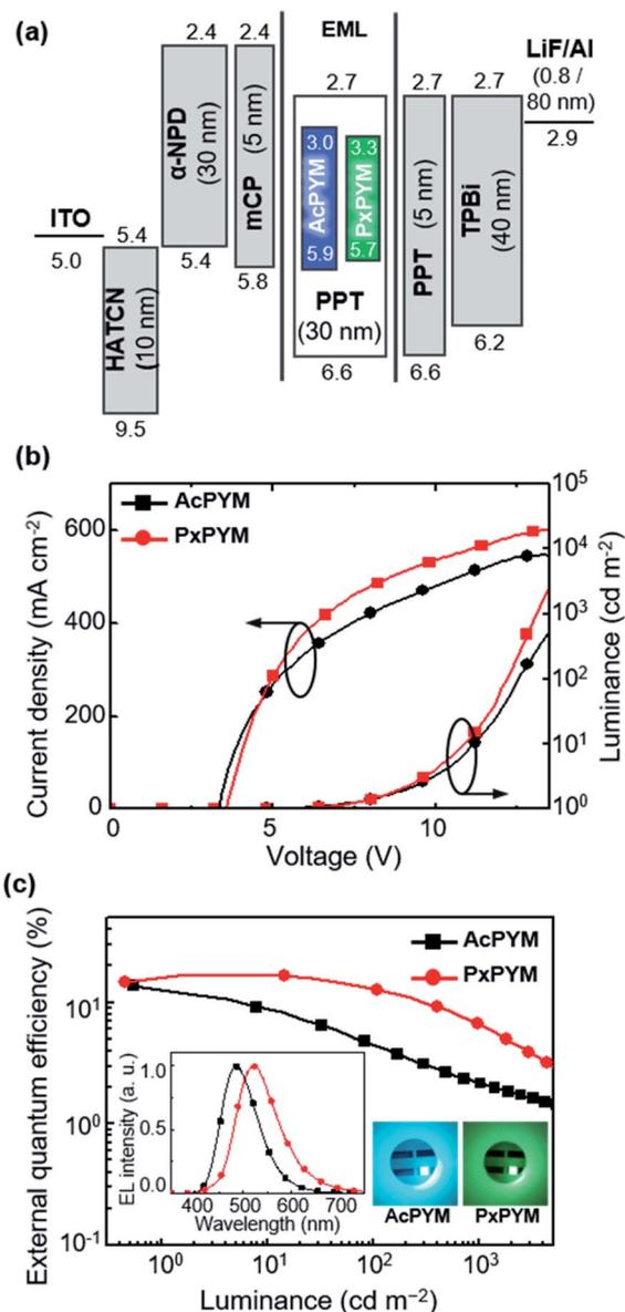
Fig. 5 (a) Energy level diagrams, (b) current density–voltage–luminance ( $J$ – $V$ – $L$ ) curves, and (c) external quantum efficiency ( $\eta_{\text{ext}}$ ) versus luminance plots of the devices employing AcPYM or PxBYM (inset: EL spectra at 10 mA cm<sup>-2</sup> and light-emitting images under electrical excitation).
