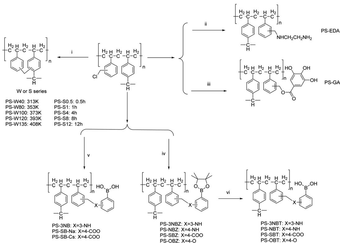
Reagents and conditions: (i) NB, AlCl<sub>3</sub>, Heat; (ii) DMF, K<sub>2</sub>CO<sub>3</sub>, EDA, 353K, 24h; (iii) DMF, NaHCO<sub>3</sub>, GA, 353K, 24h; (iv) and (v) DMF, NaHCO<sub>3</sub> or CsCO<sub>3</sub>, 353K, 24h; (vi) MeOH, NH<sub>4</sub>Cl, NaIO<sub>4</sub>, 298K, 18h.
