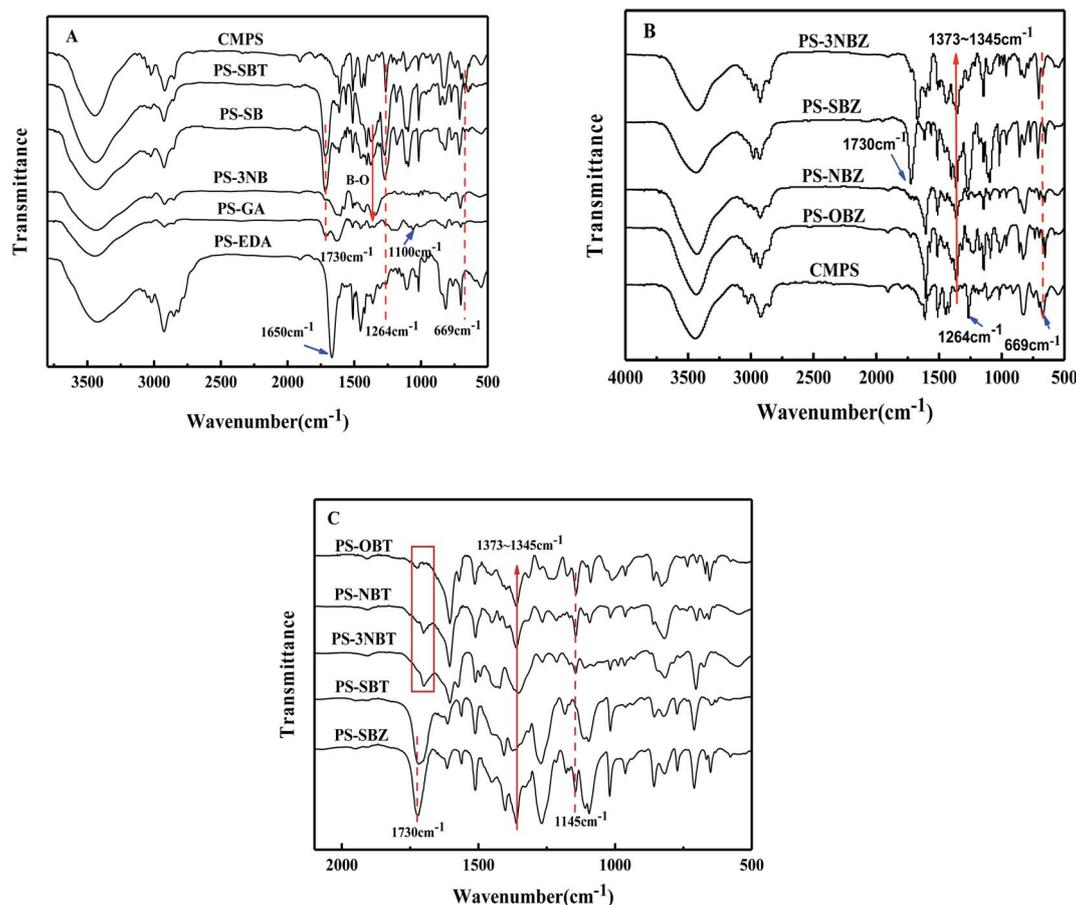
Fig. 5 IR spectra (wavenumbers from 500–4000  $\text{cm}^{-1}$ ) of modified resins with nitrogen, oxygen and boron functional groups (A), PS-SBZ type modified resins (B) and deprotection PS-SBT type modified resins (C).
