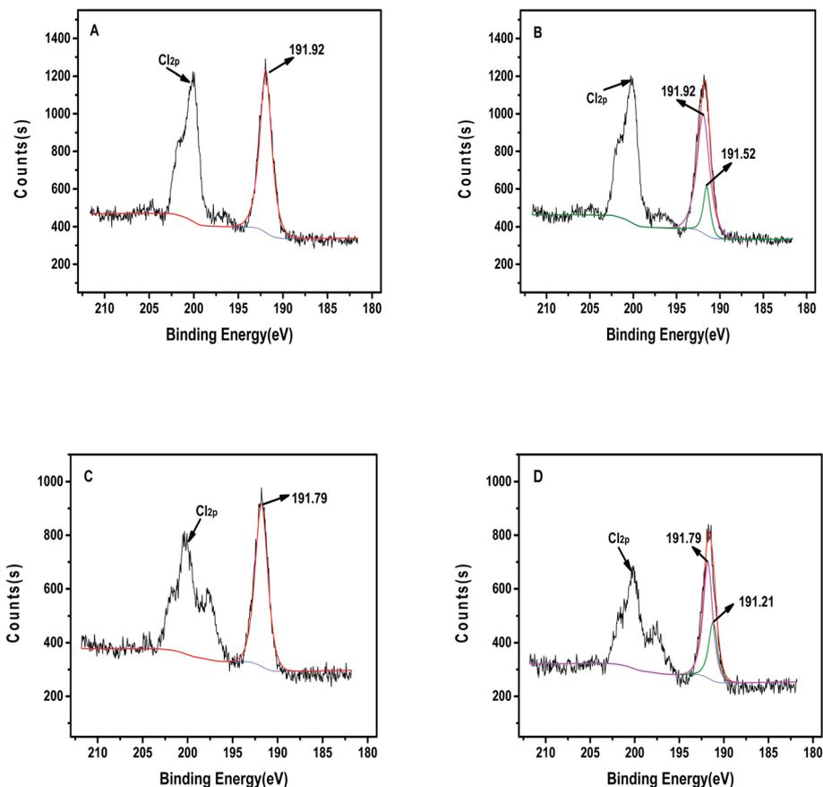
Fig. 10 XPS high resolution boron ( $B_{1s}$ ) spectra of: (A)  $B_{1s}$  before adsorption 1,3-propanediol in PS-SBT; (B)  $B_{1s}$  after adsorption 1,3-propanediol in PS-SBT; (C)  $B_{1s}$  before adsorption 1,3-propanediol in PS-3NB; (D)  $B_{1s}$  after adsorption 1,3-propanediol in PS-3NB.
