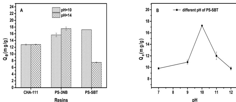
Fig. 7 Adsorption capacities of CHA-111 and boronic acid modified resins for 1,3-propanediol ((A) initial concentration  $2 \text{ g L}^{-1}$ ,  $30 \text{ }^\circ\text{C}$ , 16 h) and adsorption for 1,3-propanediol at different pH environments of PS-SBT (B) initial concentration  $2 \text{ g L}^{-1}$ ,  $30 \text{ }^\circ\text{C}$ , 16 h).
