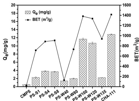
Fig. 4 Adsorption capacities for 1,3-propanediol and BET surface area of CMPS and physical resins (initial concentration 2 g L<sup>-1</sup>, 30 °C, 16 h).
