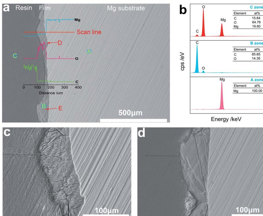
Fig. 7 Cross-sectional observations of the pure Mg carbonated in gaseous phase  $\text{CO}_2$  for 12 h: (a) SEM including an inset of the EDS line scan along the red scan line, (b) EDS analysis for zones A, B and C in (a), (c) and (d) magnified view of the selected regions in zones D and E, respectively.
