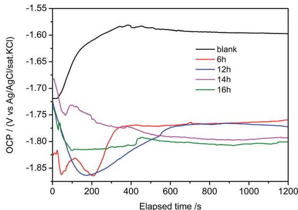
Fig. 9 Open-circuit potential evolution of the untreated and treated pure Mg samples in gaseous phase CO<sub>2</sub> during immersion in 3.5 wt% NaCl solution.
