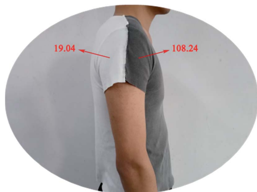
Fig. 12 The side photo of the model wearing T-shirt containing 1.25% GO (75% macro/25% superfine).
