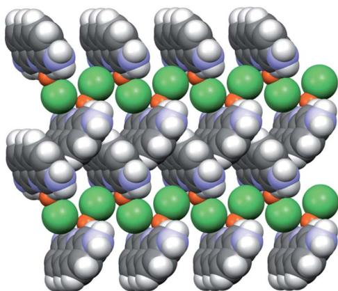
Fig. 1 Relevant packing features in crystalline PF·CuCl (**1a**), showing the herring-bone arrangement of the proflavine molecules and the 1D (CuCl···CuCl···)<sub>n</sub> chains.
