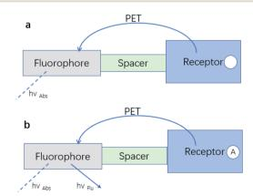
Fig. 6 (a) An electron transfer from the analyte-free receptor to the photo-excited fluorophore creates the "off" state of the sensor. (b) The electron transfer from the analyte-bound receptor is blocked resulting in the "on" state of the sensor.<sup>33</sup> (Picture from ref. 33).
