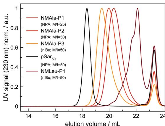
**Fig. 3** HFIP-GPC elugrams of NMAla-P1 to P3, NMLEu-P1 and polysarcosine for reference. For all the samples, toluene was used as the internal standard (peak at 23.4 mL) and polymerizations were carried out in anhydrous DMF.
