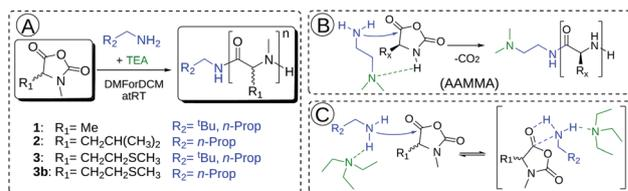
**Fig. 2** Polymerization of  $\alpha$ NNCAs **1**, **2**, **3** and **3b** in DMF (DCM) using different initiators (*n*-butyl amine and neopentyl amine) (A). Proposed accelerated amine mechanism through monomer activation (AAMMA) (B). Proposed mechanism for initiator activation caused by the added tertiary amine (TEA) (C).<sup>35</sup>
