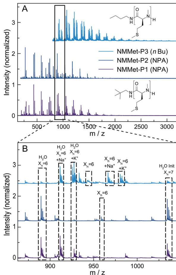
**Fig. 6** Full MALDI-ToF spectra of NMMet-P1 (lower, purple), NMMet-P2 (middle, dark blue) and NMMet-P3 (upper, light blue) (A) and the corresponding magnifications (B) with assignment of the individual peaks.
