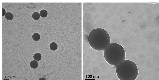
**Fig. 2** TEM images of PSt latex particles synthesized in the presence of MgAl-LDH nanoparticles at low and high magnification, showing the absence of interaction between the two populations of particles (St1 in Table 1).
