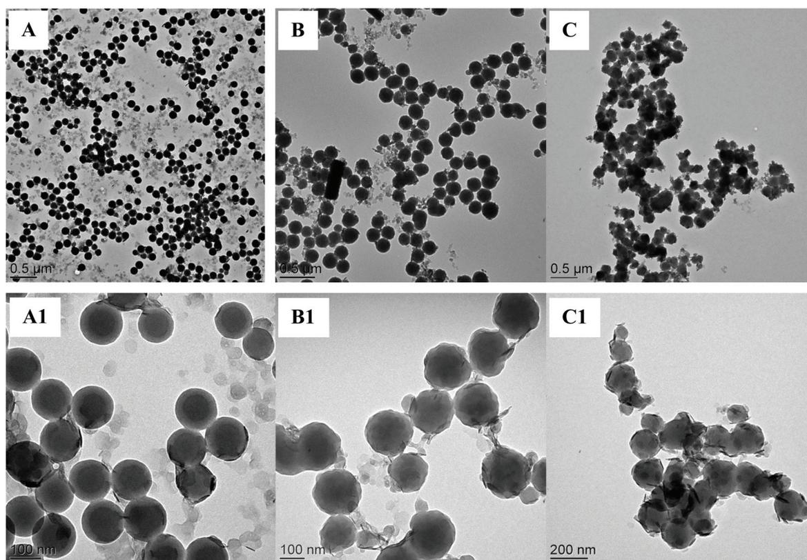
**Fig. 3** TEM images of LDH/polymer composite particles obtained by Pickering emulsion copolymerization of St and HEMA in the presence of 10 wt% of LDH (based on total monomer) for increasing HEMA contents: (A and A1) 4.0 wt%, (B and B1) 8.0 wt% and (C and C1) 12.0 wt%, based on total monomer (runs H02, H04 and H05 in Table 1).
