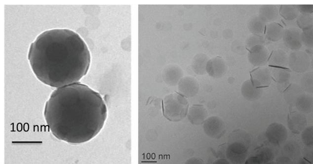
**Fig. 7** TEM (left) and cryo-TEM (right) images of LDH/polymer composite latex particles obtained by Pickering emulsion copolymerization of St and MMA (St/MMA = 80/20 wt/wt) in the presence of 10 wt% of LDH (M02 in Table 2). More images can be seen in the ESI (Fig. S3†).
