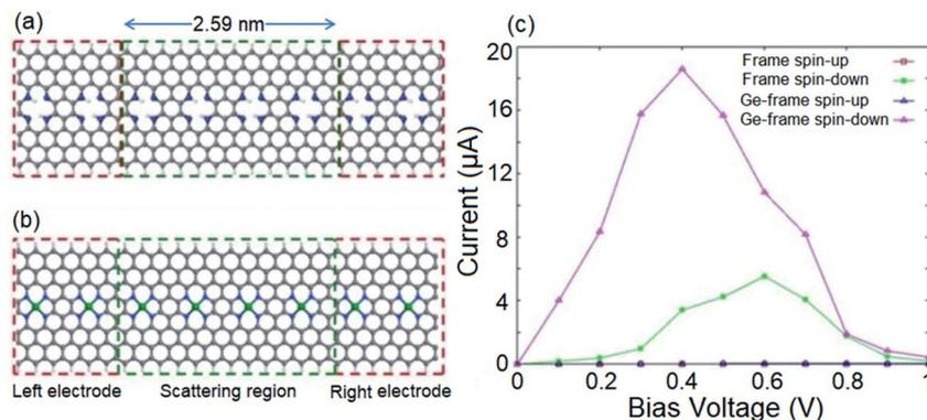
Fig. 4 Schematic illustrations of the proposed two-probe systems for (a) hydrogenated and (b) Ge-doped systems.  $n = 8$  ZGNR is used for both scattering and semi-infinite electrode regions. (c) Spin resolved current–voltage profiles of hydrogenated and Ge-doped transport systems.
