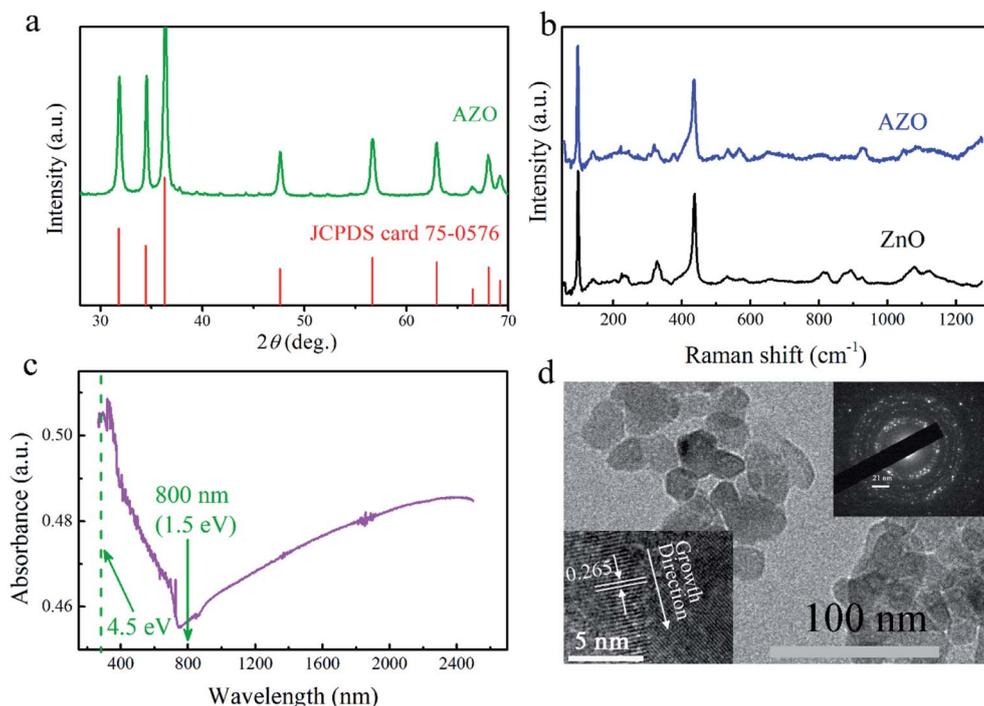
**Fig. 1** Characteristics and linear optical properties of the obtained AZO NCs. (a) X-ray diffraction (XRD) pattern of the as-prepared AZO NCs. Here, for clarity, the JCPDS card (JCPDS# 75-0576) is shown as a reference. (b) Raman spectrum excited using a laser of 532 nm. (c) Linear optical absorption of AZO NCs. (d) Low-magnification TEM image, the SAED pattern (upper-right in the inset), and high-resolution TEM image (lower-left in the inset).
