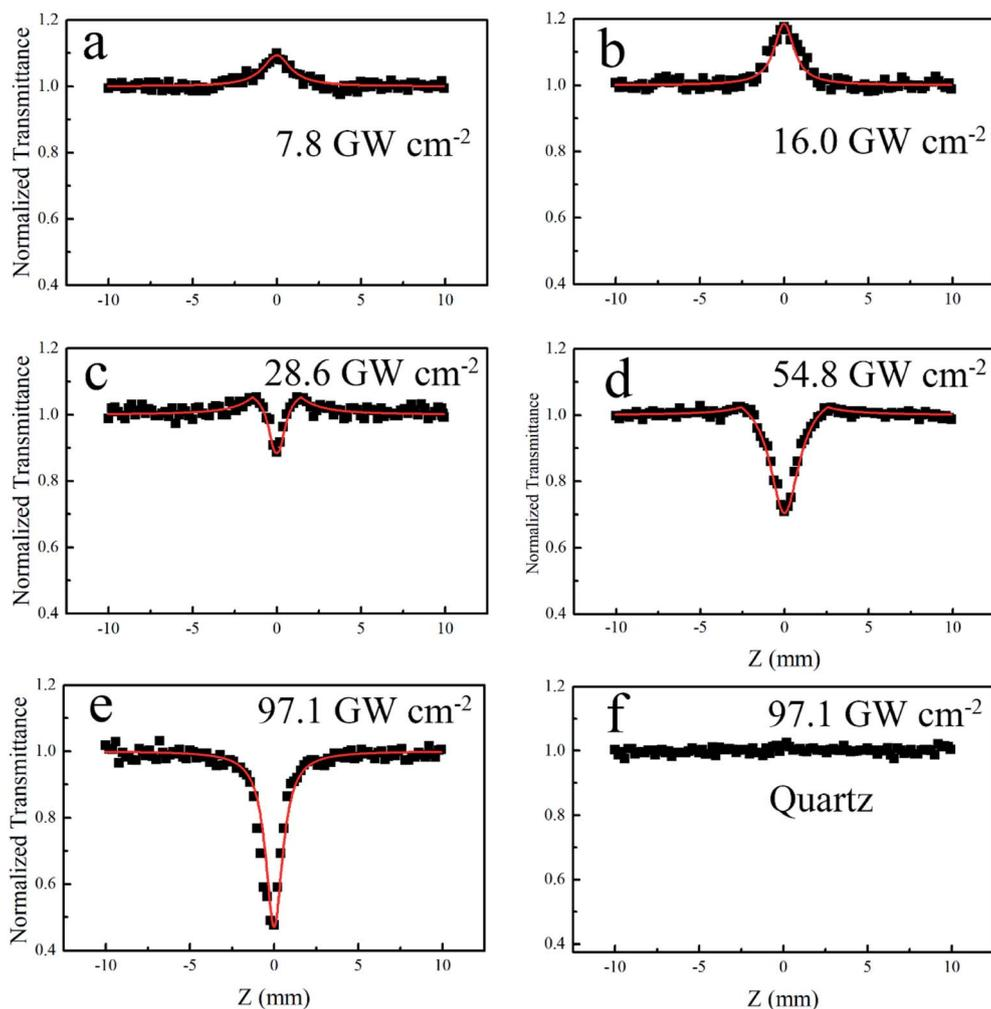
Fig. 2 Open Z-scan results (black square) and fitting curves (red line) of the AZO/quartz film measured by using a pump source of 800 nm-laser at different pulse intensities: (a)  $7.8 \text{ GW cm}^{-2}$ , (b)  $16.0 \text{ GW cm}^{-2}$ , (c)  $28.6 \text{ GW cm}^{-2}$ , (d)  $54.8 \text{ GW cm}^{-2}$  and (e)  $97.1 \text{ GW cm}^{-2}$ . (f) The blank quartz under the pulse intensity of  $97.1 \text{ GW cm}^{-2}$ .
