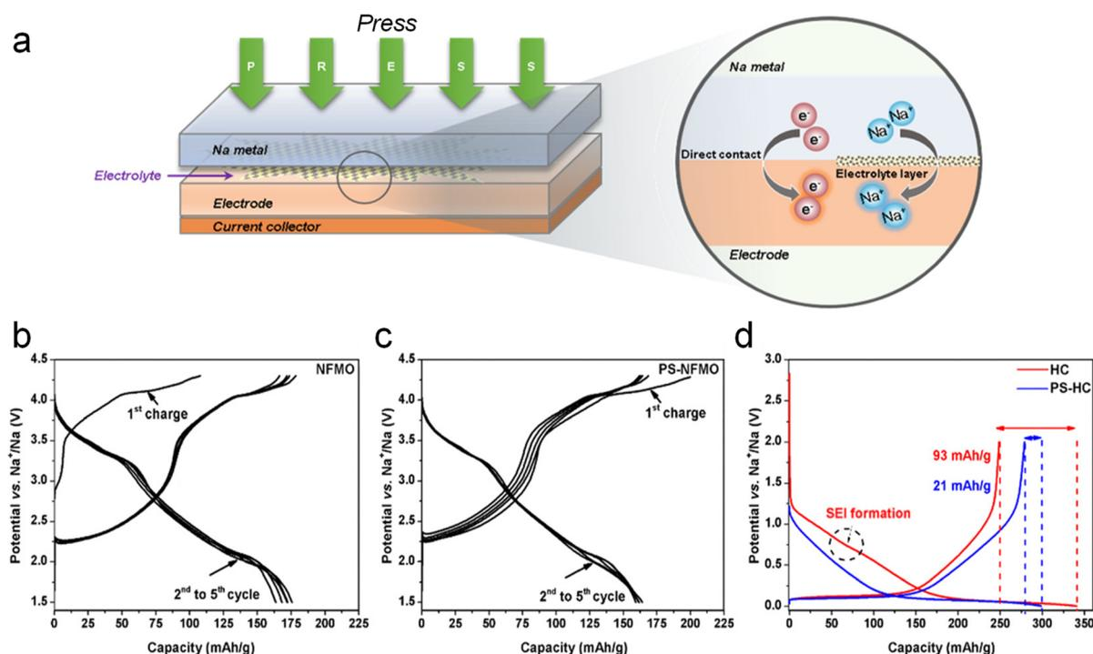
Fig. 2 (a) Schematic illustration of direct contact SCT. Charge–discharge profiles of  $\text{Na}_{0.67}\text{Fe}_{0.5}\text{Mn}_{0.5}\text{O}_2$  (b) before and (c) after sodium compensation. (d) Galvanostatic charge–discharge curves of HC electrodes with/without SCT. Reproduced with permission.<sup>30</sup> Copyright 2019, American Chemical Society.
