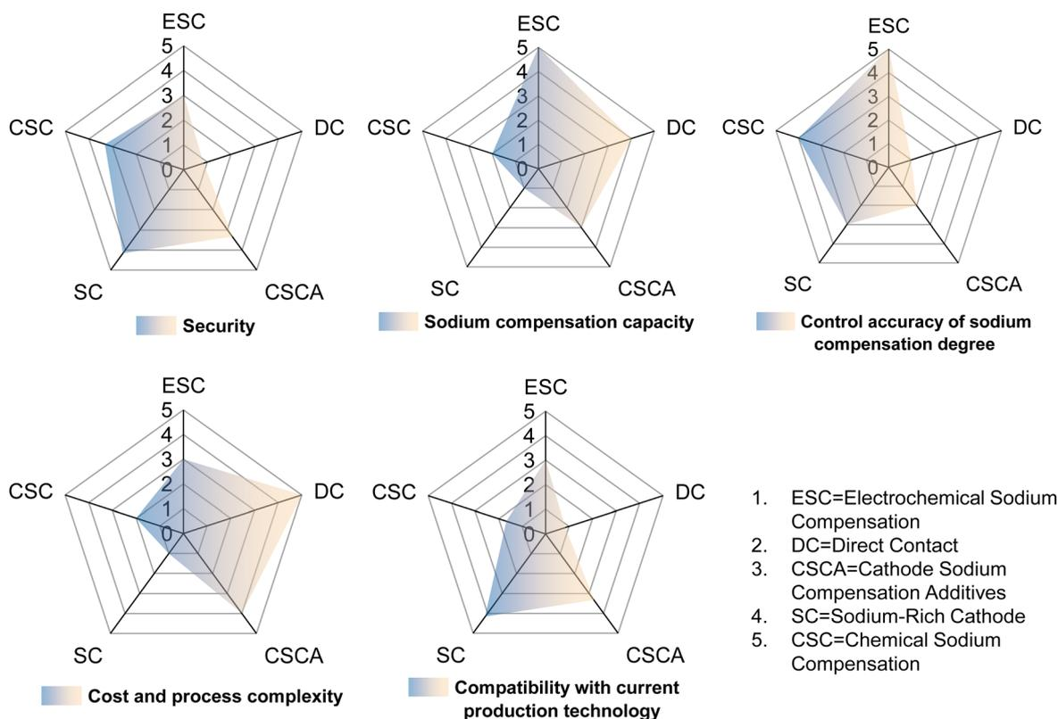
Fig. 10 Key parameter radar chart of different SCTs.
