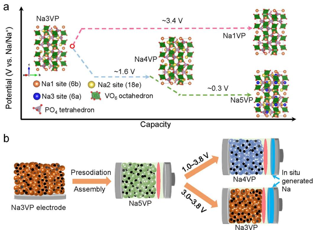
Fig. 8 (a) Schematic illustration for phase transformations of  $\text{Na}_x\text{V}_2(\text{PO}_4)_3$  and corresponding electrochemical potentials. (b) Illustration of sodium compensation on  $\text{Na}_x\text{V}_2(\text{PO}_4)_3$ , battery assembly, and battery operation within two different voltage windows. Reproduced with permission.<sup>81</sup> Copyright 2022, Wiley-VCH.
