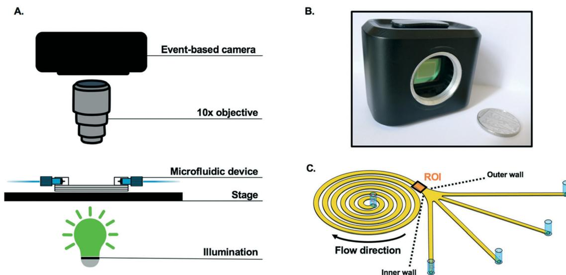
Fig. 2 Imaging in inertial focusing devices. A. Illustration of the optical setup. Experiments were performed with a standard fluorescent microscope, with the event-based camera mounted *via* a C-mount port. B. Picture of the event-based camera used in this work. The camera is circa 5.7 cm in width, 4.8 cm in height and 3.6 cm in depth. C. Schematic of the spiral channel used for focusing experiments with images recorded in the region of interest (ROI).
