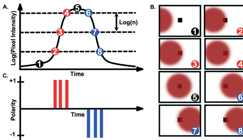
**Fig. 1** Event-based detection of a particle over time. A. Represents the light flux reaching a given pixel when a fluorescent particle passes through the pixel field of view (B). C. When the light intensity change (with respect to the last recorded event) exceeds a user-defined threshold, the camera records a new event whose polarity encodes the sign of the intensity change.
