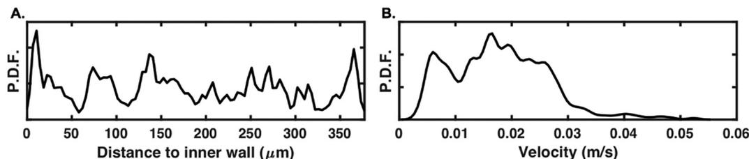
Fig. 8 Tracking results of 1  $\mu\text{m}$  fluorescent particles at  $U_f = 0.04 \text{ m s}^{-1}$ . Probability density functions (P.D.F.) of A. tracked particles as a function of the distance to the spiral inner wall and B. corresponding particle velocities. Plots A and B are based on particles tracked in the blue region of interest highlighted in Fig. 7A.
