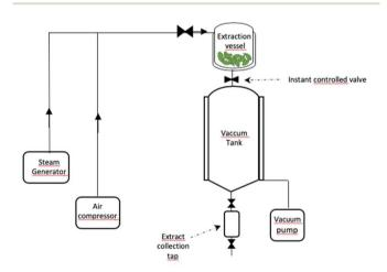
Fig. 2 Simplified schematic representation of DIC equipment.
