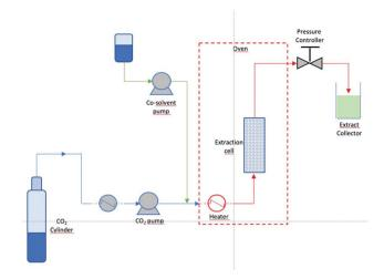
Fig. 3 Simplified schematic representation of supercritical CO<sub>2</sub> equipment.
