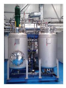
Fig. 4 Lab and industrial scale liquefied gas extraction systems from CELSIUS-France
