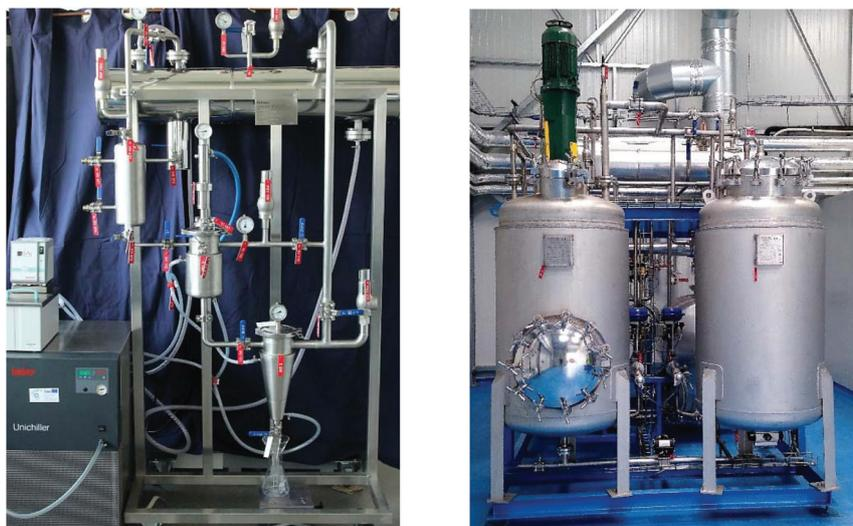
Fig. 4 Lab and industrial scale liquefied gas extraction systems from CELSIUS-France.
