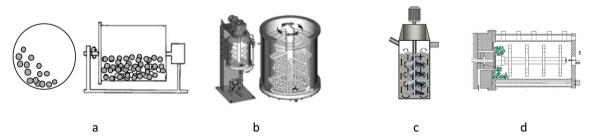
Fig. 6 Development of agitated mills (a), ball mills; attritors (b, 1928); 2 sand mills "Sand Mills" (c; 1950); 3 agitated disc mills (d). 71
