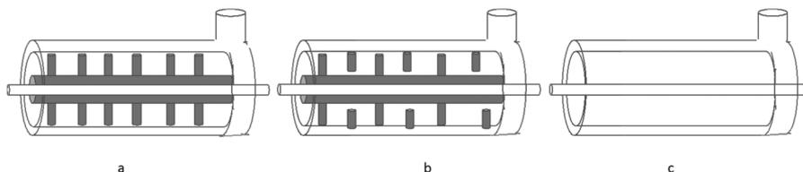
Fig. 7 Different ball mill geometries (a) agitating disc mills; (b) finger to finger mills; annular gap mill (c).<sup>71</sup>
