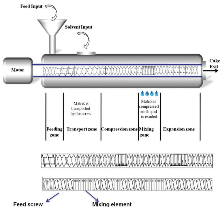
Fig. 5 Example of unitary actions in an extruder.
