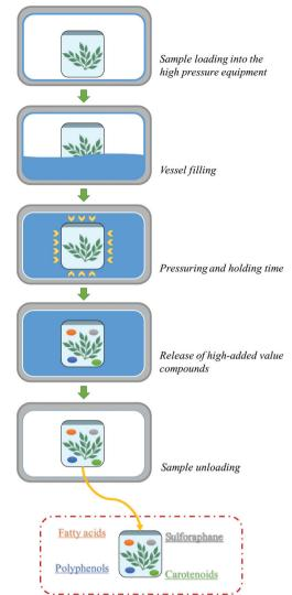
Fig. 11 Schematic representation of extraction assisted by higher pressure.
