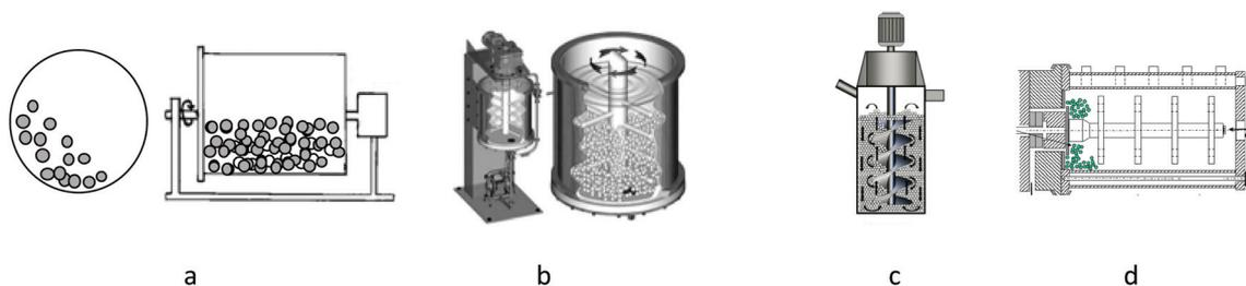
Fig. 6 Development of agitated mills (a), ball mills; attritors (b, 1928);<sup>72</sup> sand mills "Sand Mills" (c; 1950);<sup>73</sup> agitated disc mills (d).<sup>71</sup>
