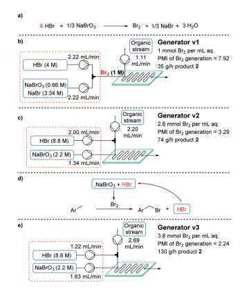
Fig. 3 Summary of three "generations" of  $Br_2$  generator, including their flow setup, PMI of  $Br_2$ , aqueous volume efficiency and productivity in the conversion of 1 to monobrominated product 2. The displayed flow rates show the required values for a residence time of 30 s.
