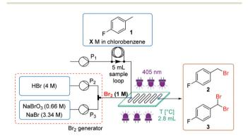
Fig. 2 Initial experimental setup using 1<sup>st</sup> generation Br<sub>2</sub> generator.
