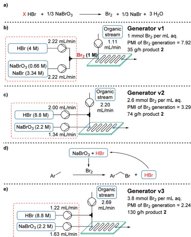
Fig. 3 Summary of three “generations” of Br<sub>2</sub> generator, including their flow setup, PMI of Br<sub>2</sub>, aqueous volume efficiency and productivity in the conversion of **1** to monobrominated product **2**. The displayed flow rates show the required values for a residence time of 30 s.
