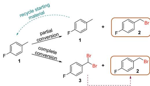
Fig. 5 Scheme showing the complementary approaches to obtaining optimal productivity of desired product 2, by starting material recycling, or diethyl phosphite reduction.
