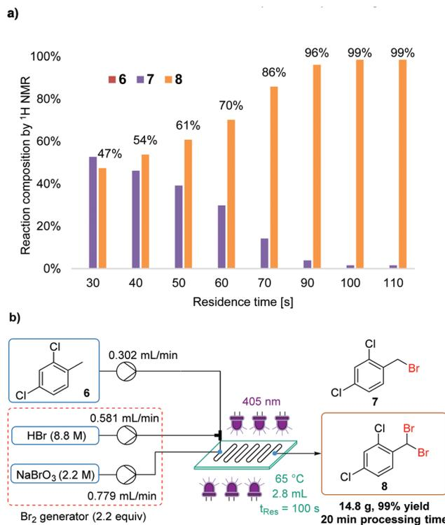
Fig. 8 (a) Graph showing the effect of residence time upon the mono- (**7**) to dibrominated (**8**) product ratio; (b) experimental setup using 3<sup>rd</sup> generation Br<sub>2</sub> generator for the synthesis of 2,4-dichlorobenzyl bromide **8**.
