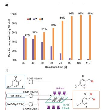
Fig. 8 (a) Graph showing the effect of residence time upon the mono-(7) to dibrominated (8) product ratio; (b) experimental setup using 3rd generation Br2 generator for the synthesis of 2,4-dichlorobenzal bromide 8.
