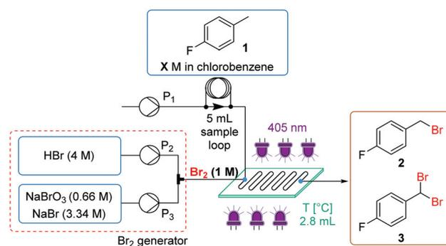
Fig. 2 Initial experimental setup using 1<sup>st</sup> generation  $\text{Br}_2$  generator.
