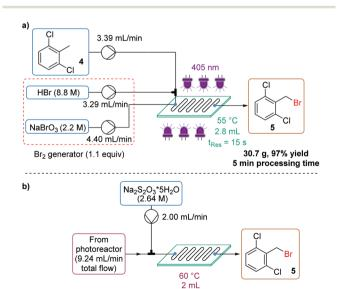
Fig. 7 (a) Schematic representation of the experimental setup for the synthesis of 2,6-dichlorobenzyl bromide 5 using the 3<sup>rd</sup> generation Br<sub>2</sub> generator; (b) schematic representation of the in-line sodium thiosulfate quench setup, ensuring that no Br2 remains.
