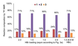
Fig. 4 Chart showing the performance of benzylic bromination upon altering equivalents of HBr used in the bromine generator.
