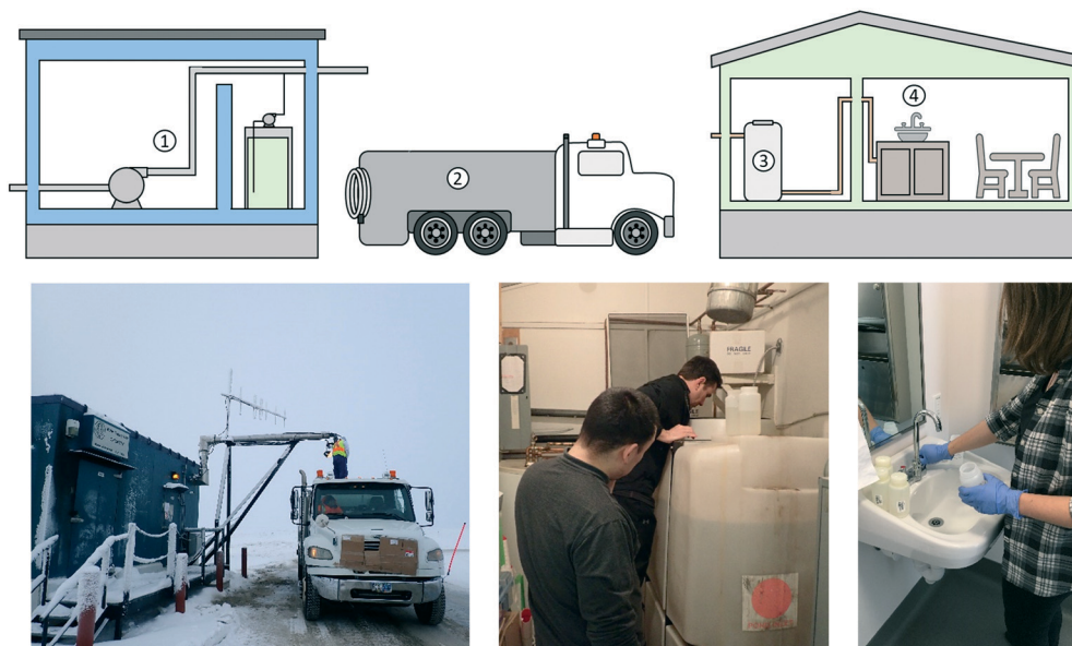
Fig. 1 Trucked drinking water system in Pond Inlet, NU. Water is pumped from Water Lake (1) and chlorinated as it is transferred to the truck (2). The truck delivers the water to individual buildings, where it is stored onsite in a domestic water storage tank (3) until it is required at the point of use (4).
