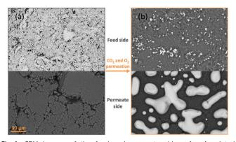
Fig. 1 SEM images of the feed and permeate sides of a Ag-plated dual-phase  $Al_2O_3$ -supported membrane before and after  $CO_2$  and  $O_2$  permeation. (a) An electroless-plated layer of Ag was deposited on the feed side only. (b) Following 80 hours of  $CO_2$  and  $O_2$  permeation at 650 °C, Ag was significantly corroded on the feed side, with  $\sim$ 3% appearing on the permeate side. Feed-side inlet: 50 mol%  $CO_2$ , 25 mol%  $O_2$  and 25 mol%  $N_2$ . Permeate-side inlet: Ar.
