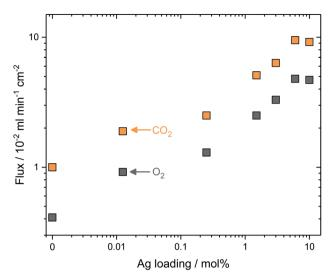
Fig. 3 Effect of Ag loading on  $CO_2$  and  $O_2$  fluxes at 650 °C. Stable  $CO_2$  and  $O_2$  fluxes (defined as a minimum of 4 hours where the mean flux varied less than  $\pm 3\%$ ) for dual-phase membranes with Ag powder loaded into molten carbonate. The standard deviation in flux during 4 hours was smaller than the data-point symbols used. Feed-side inlet: 50 mol%  $CO_2$ , 25 mol%  $O_2$  and 25 mol%  $N_2$ . Permeate-side inlet: Ar.
