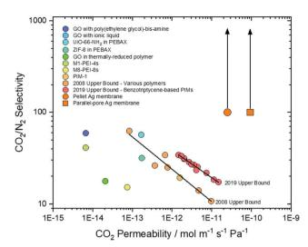
State-of-the-art membrane comparison. Graphene oxide, mixed-Fia. 7 matrix, SPONG and polymer membranes, with the 2008 and 2019 upper bounds. Pellet and parallel-pore Ag membranes are shown with minimum selectivity ( $\sim 100$ ) calculated by assuming N<sub>2</sub> permeation at the limit of detection of the analytical apparatus used (no N2 was detected at the permeate-side outlet). This selectivity may be as high as >1000 if considered on the basis of CO<sub>2</sub>/N<sub>2</sub> solubility.
