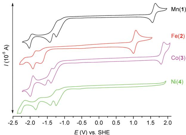
Fig. 9 Cyclic voltammograms of complexes **1** (black), **2** (red), **3** (purple), and **4** (green) ( $\sim 2$  mM) recorded under an argon atmosphere in 0.1 M TBAP in acetonitrile with a glassy carbon working electrode. Complex **2** was the only one used for the measurement in its form prior to recrystallization from  $\text{CH}_3\text{NO}_2$ .
