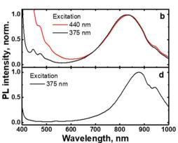
Fig. 6 (a): Normalized absorption and PLE spectra of (C6)-(2)-SiNc; (b): PL spectra of (C6)-(2)-SiNc at different excitation wavelengths. The edge of emission of LEDs used for excitation is observed at  $\lambda$  < 500 nm; (c): normalized absorption and PLE spectra of (C6)-(3)-SiNc; (d): PL spectra of (C6)-(3)-SiNc excited at 375 nm. The edge of emission of LED used for excitation is observed at  $\lambda$  < 400 nm. PLE spectra were measured at the emission wavelength of 800 nm.
