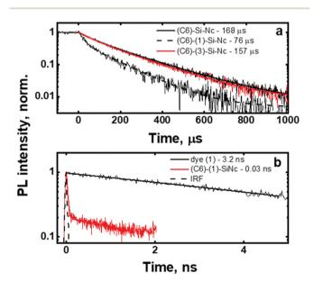
Fig. 4 (a): Long-time (μs) PL decays for ligand functionalized SiNc excited at 405 nm and measured at 810 nm. (b): Short-time (ns) PL decays of dye (1) and (C6)-(1)-SiNc; excited at 440 nm and measured at 450-550 nm. IRF is the instrument response function.
