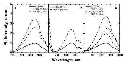
Fig. 5 (a): PL under excitation with LED440 nm of (C6)-SiNc, (C6)-(1)-SiNc and (C6)-(2)-SiNc; (b): PL under excitation with LED 515 nm of (C6)-SiNc and (C6)-(3)-SiNc; (c): PL under broadband excitation (435-550 nm) of (C6)-SiNc, (C6)-(1)-SiNc, (C6)-(2)-SiNc and (C6)-(3)-SiNc. All dispersions have similar absorbance of 0.3 at 300 nm ( $A_{300}$ ). The PL spectra were normalized to emission of (C6)-SiNc.
