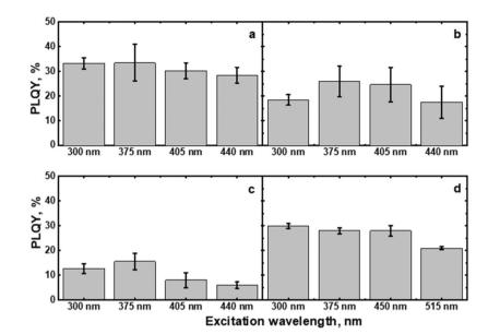
Fig. 3 PLQY values of (a): (C6)-SiNc, (b): (C6)-(1)-SiNc, (c): (C6)-(2)-SiNc and (d): (C6)-(3)-SiNc measured at different excitation wavelengths. The PLQY values are the result of averaging for five independent synthetic batches. The error bars indicate maximum and minimum values measured for five independent synthetic batches.
