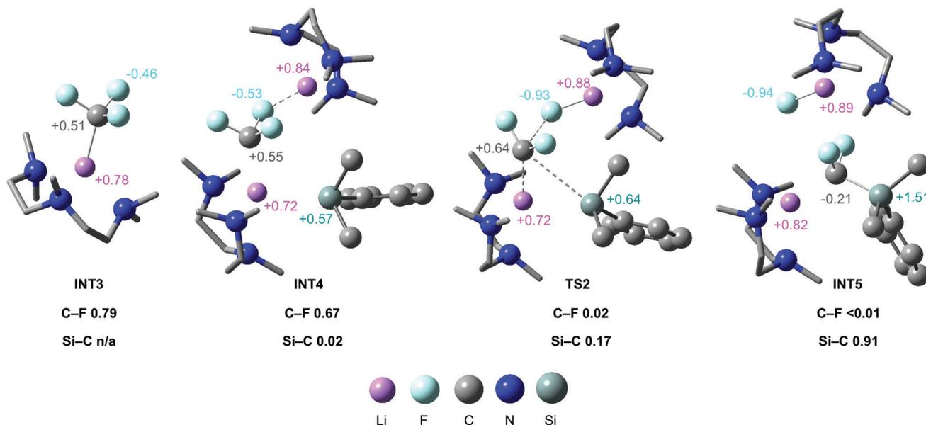
Fig. 5 Calculated structures for the stationary points of the C–F activation step, annotated with relevant NPA charges and Wiberg Bond Indices for C–F cleavage and C–Si formation.
