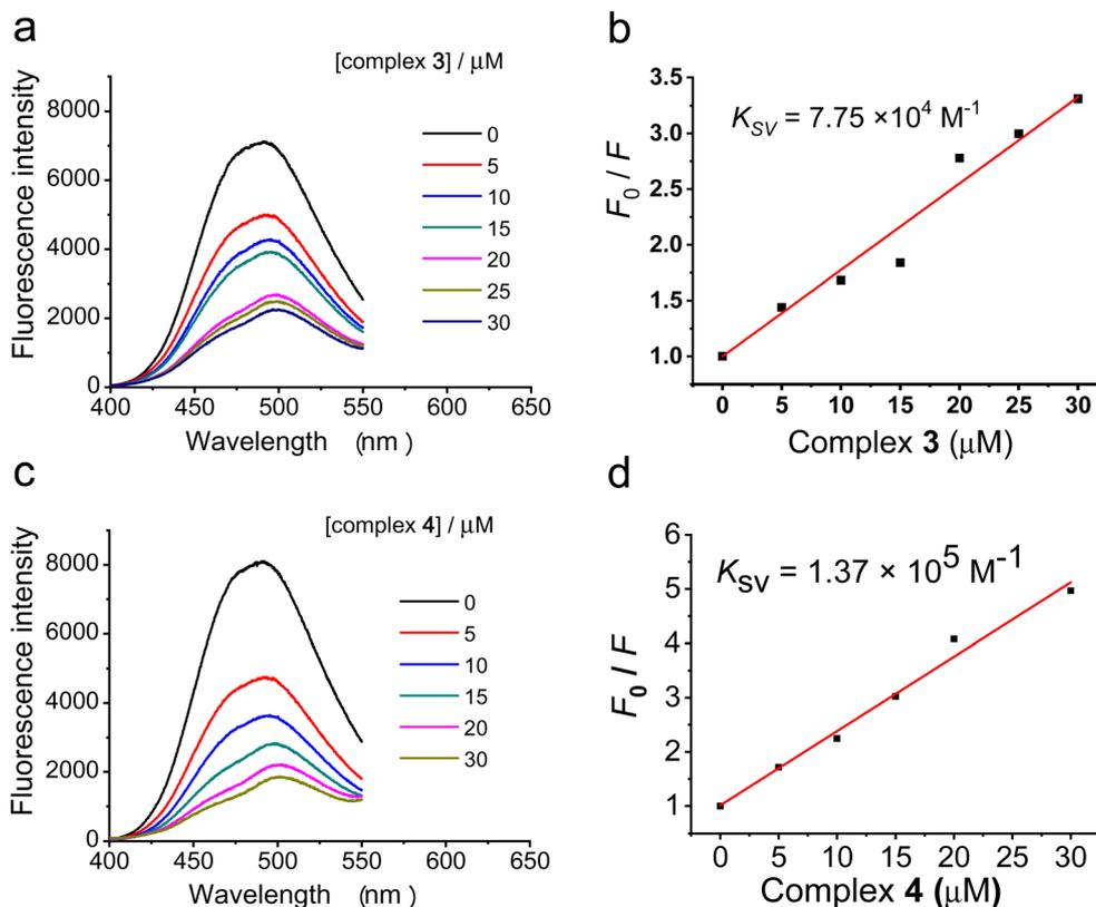
**Fig. 4** Competitive displacement assay. (a and c) Fluorescence titration of the Hoechst-ctDNA complex with complexes 3 and 4, respectively, in Tris buffer (Hoechst: ctDNA = 20 : 200  $\mu\text{M}$ ) at  $\lambda_{\text{ex}} = 370 \text{ nm}$ . (b and d) The corresponding Stern-Volmer plot for the quenching of fluorescence intensity at 488 nm upon the addition of complexes 3 and 4, respectively.
