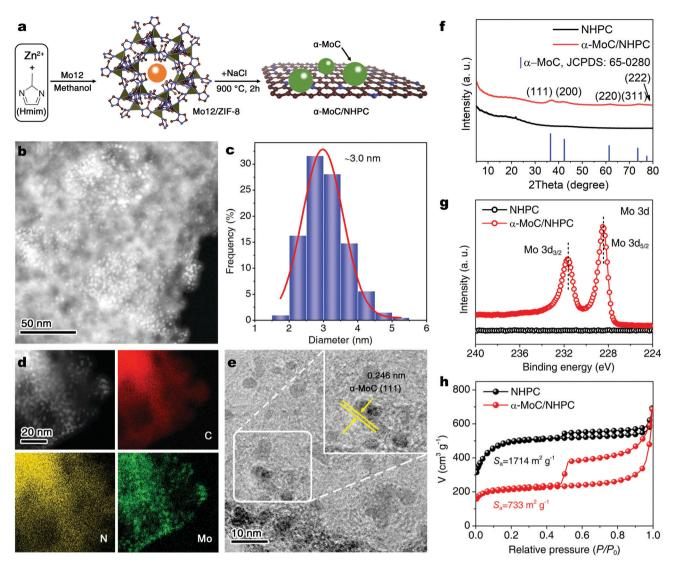
(a) Schematic illustration of the synthesis of  $\alpha$ -MoC/NHPC. (b) HAADF-STEM image of  $\alpha$ -MoC/NHPC and (c) the corresponding  $\alpha$ -MoC NPs size distribution. (d) Elemental mapping images showing the distribution of C (red), N (yellow), and Mo (green) elements. (e) HRTEM image of  $\alpha$ -MoC/NHPC. (f) XRD patterns, (g) high-resolution Mo 3d XPS spectra, (h) N<sub>2</sub> adsorption/desorption isotherms of NHPC and α-MoC/NHPC.
