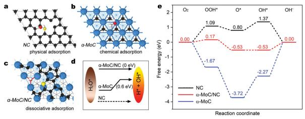
Fig. 3 Adsorption configurations of water on (a) NC, (b) α-MoC(111) and (c) α-MoC/NC surfaces. (d) Schematic energy diagrams for water dissociation and (e) free energy diagrams for ORR on NC,  $\alpha$ -MoC(111) and  $\alpha$ -MoC/NC catalysts at the overpotential of 0 V.
