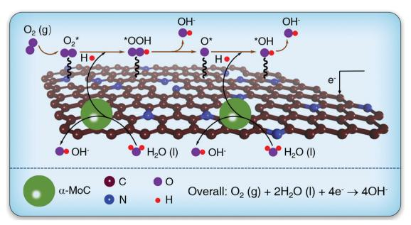
Scheme 1 Schematic illustration for water dissociation step and the subsequent elementary processes for ORR in alkaline solutions over an  $\alpha$ -MoC/ NHPC electrocatalyst
