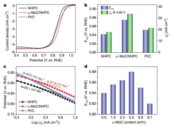
Fig. 2 (a) ORR polarization curves, (b)  $J_k$  at 0.80 V and  $E_{1/2}$ , and (c) corresponding Tafel slopes of NHPC, α-MoC/NHPC and Pt/C. (d)  $E_{1/2}$  of α-MoC/NHPCs with different α-MoC contents.
