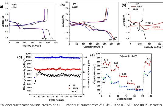
Fig. 4 Initial discharge/charge voltage profiles of a Li-S battery at current rates of 0.05C using (a) PVDF and (b) PP separator. Also (c) galvanostatic discharging/charging performance of Li-S batteries with different separators at 0.05C and (d) cycling performance of the Li-S batteries with different separators at 0.1C, (e) rate capability performance of Li-S batteries with different separators at various current rates ranging from 0.1 to 2C, and returning to 0.1C
