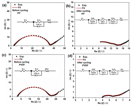
Fig. 5 Nyquist plots for LSB cells before and after cycling with (a), (b) PP and (c), (d) PVDF separators. The equivalent circuit parameters: R-e = electrolyte resistance, R-ct = charge-transfer resistance, R-SEI = resistance of solid electrolyte interphase, R-film related to Li<sub>2</sub>S/Li<sub>2</sub>S<sub>2</sub> film, and Ws. CPE-ct, CPE-sd, CPE-SEI and CPE-film represent constant phase elements associated with R-ct, R-SEI and R-film respectively
