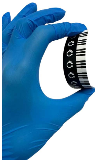
Fig. 4 Screen-printed sensors produced on flexible substrate.
