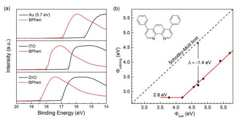
Fig. 1 (a) Photoemission cutoff for the secondary electrons of various substrates with and without BPhen. (b) Summary of the  $\Phi_{\text{sub/org}}$  changing with  $\Phi_{\text{sub}}$ . The fitting line (red) follows well with the ICT model except for a negative displacement ( $\Delta$ ). The inset shows the molecular structure of BPhen.
