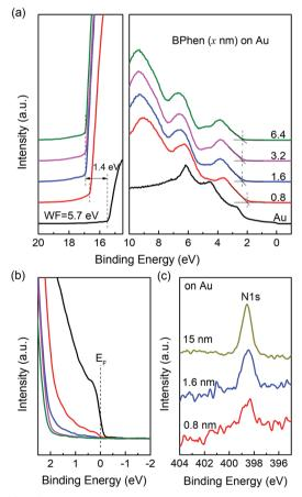
Fig. 2 (a) UPS spectra of Au with incrementally deposited BPhen layer. (b) Magnifications of the same spectra near the Fermi level. (c) XPS spectra of BPhen on Au with different thickness. From the spectra we confirmed the large dipole only occurs in the first layer and there is no band bending or chemical interaction near the interface
