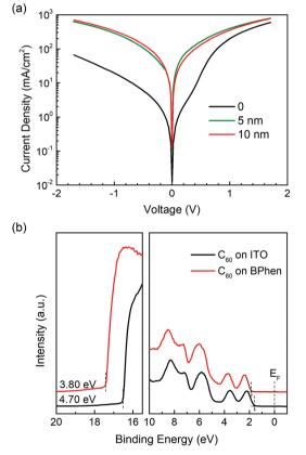
Fig. 5 (a) Current density-voltage characteristics of ITO/BPhen/C<sub>60</sub>/LiF/Al electron-only device with varying BPhen thickness. Negative bias corresponds to electron injecting from ITO side. (b) Comparison of UPS spectra for C<sub>60</sub> on ITO and ITO/BPhen.
