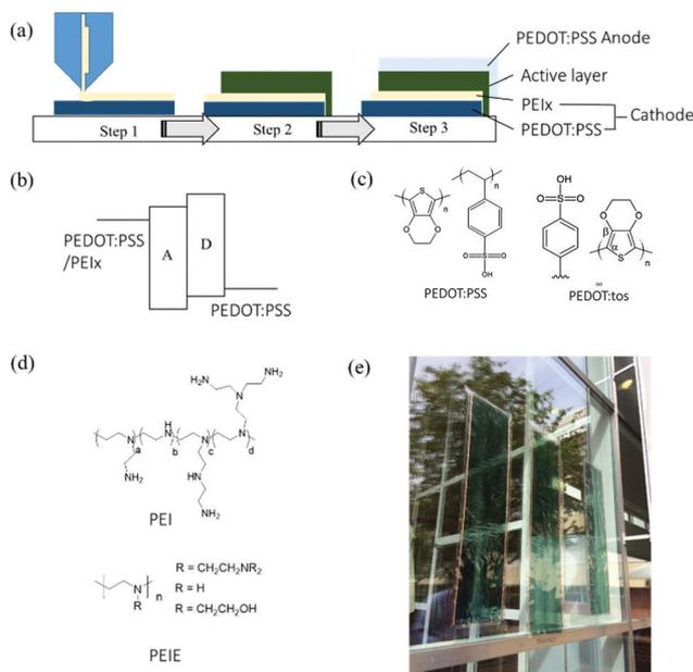
**Fig. 1** (a) Schematic of PEI layer coated on PEDOT:PSS layer with slot die coating and the device printing process (3 steps). (b) Energy diagram of printed solar cells, A: electron acceptor, D: electron donor. (c) Chemical structures of PEDOT:PSS, PEDOT:tos and (d) PEI and PEIE. (e) Printed large area modules using the developed device structure and fabrication method reported in this work, photographed by the author.
