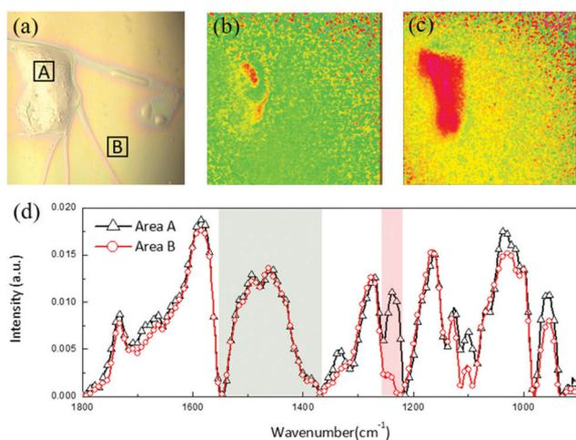
**Fig. 5** Polar solvent removes and redistributes free PSS in highly conductive PEDOT:PSS electrodes. (a) Reflection mode optical microscopy. Relative absorption mapping of (b) the C=C stretching from PEDOT (integrated from 1500–1400 cm<sup>-1</sup>) and (c) the -S=O stretching in PSS (integrated from 1282–983 cm<sup>-1</sup>) from a PEDOT:PSS film where water has been deposited and left to evaporate. (d) IR spectra of areas A and B in (a).
