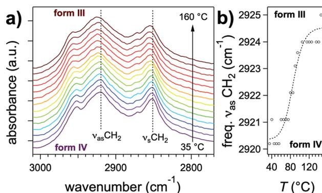
Fig. 6 (a) Evolution of the FTIR spectrum in the CH stretching area upon transition from the crystalline form IV to the lamellar phase III. (b) Position of the  $\nu_{\text{as}}\text{CH}_2$  band as a function of temperature.
