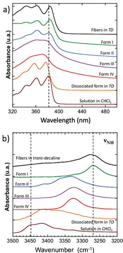
Fig. 5 (a) UV-vis spectra of the four polymorphs of NDI2 and in solution in chloroform and in *trans*-decaline (TD). The dissociated form in TD is obtained at  $T = 120$  °C. (b) FTIR spectra (thin films) of the four polymorphs of NDI2, the melt and the solutions in TD. In both plots, the successive spectra were offset along the ordinate axis for clarity.
