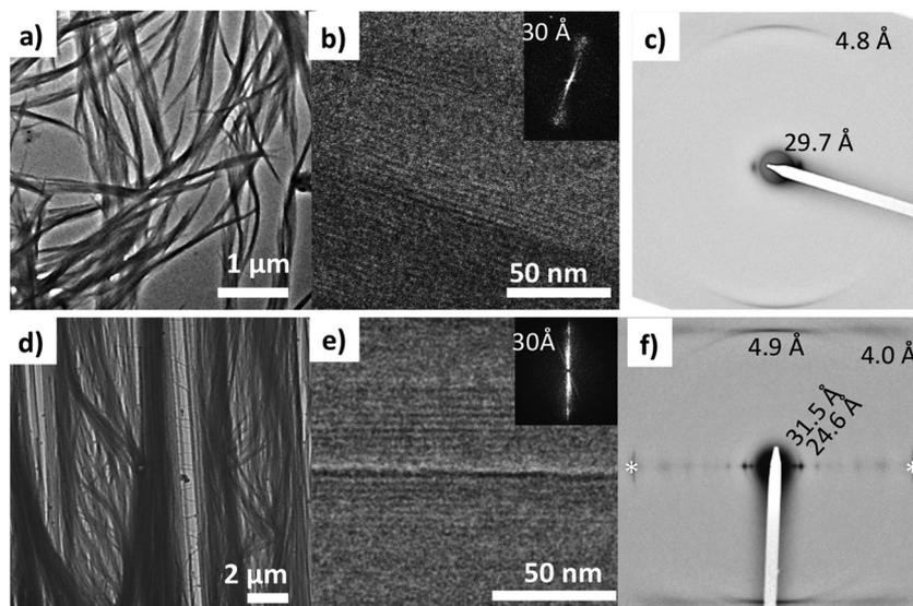
**Fig. 7** (a–c) Fibrillar morphology of NDI2 dried gel phase. (a) Bright field, (b) HRTEM with corresponding FFT, (c) electron diffraction pattern. (d–f) Morphology of oriented NDI2 films obtained by SVA in  $\text{CHCl}_3$  on oriented PTFE substrates. (d) Bright field, (e) HRTEM with corresponding FFT, (f) electron diffraction pattern. The asterisk points at the 100 reflection of the oriented PTFE substrate (4.9 Å) used as a reference to calculate reticular distances.
