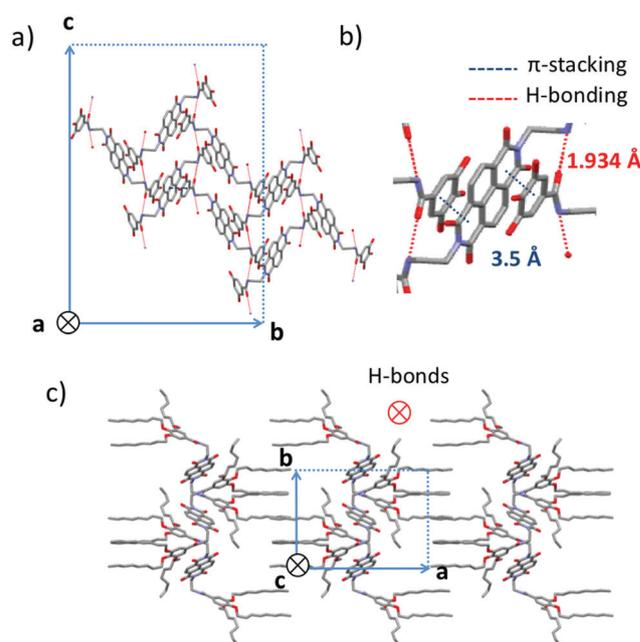
**Fig. 8** Representation of the crystal lattice of form IV of NDI2. (a) Along the  $a$  axis and (c) along the  $c$  axis. (b) Enlarged view of an NDI core  $\pi$ -stacked between two phenyl units of two adjacent dendrons. Red dotted lines show H-bonds between amide groups whereas blue dotted lines show short  $\pi$ -stacking distances.
