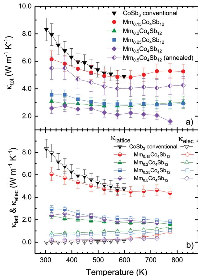
Fig. 6 Temperature dependence of the total thermal conductivity (upper panel), and electronic ( $\kappa_e$ ) and lattice ( $\kappa_l$ ) contributions (bottom panel) of  $Mm_xCo_4Sb_{12}$  and  $CoSb_3$  conventional (from ref. 16). Data for an annealed  $Mm_{0.5}Co_4Sb_{12}$  sample at 873 K have been included for comparison.
