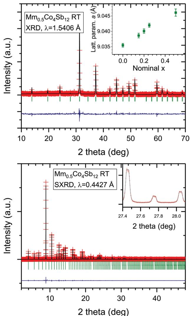
Fig. 1 Experimental points (red crosses), calculated profile (black line), difference (blue line) and Bragg reflections (green symbols). (a) laboratory XRD pattern with Cu  $K_{\alpha}$  radiation. The inset shows the variation of the a unit-cell parameter with the nominal x content, and (b) SXR pattern for  $Mm_{0.5}Co_4Sb_{12}$  at RT.
