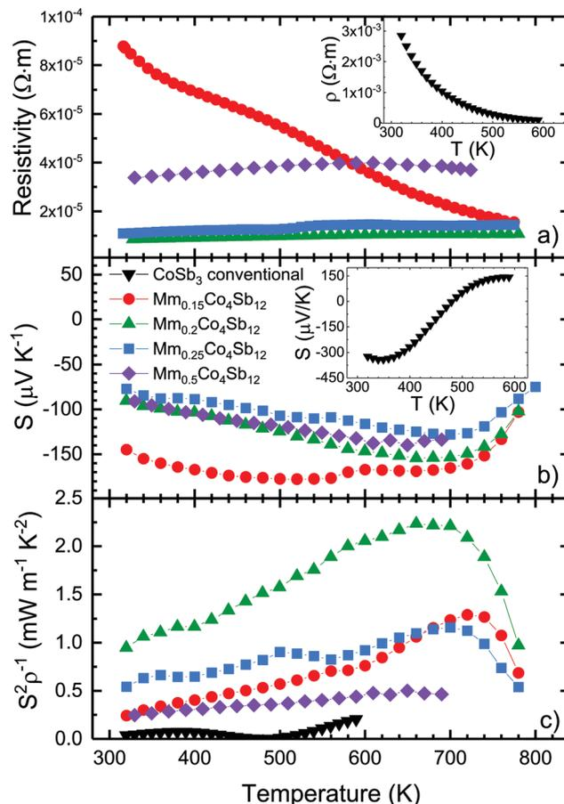
Fig. 5 Temperature dependence of the (a) electrical resistivity, (b) Seebeck coefficient ( $S$ ) and (c) power factor ( $S^2\rho^{-1}$ ) of  $Mm_xCo_4Sb_{12}$  and pure  $CoSb_3$  (insets) prepared by conventional methods (from ref. 16).
