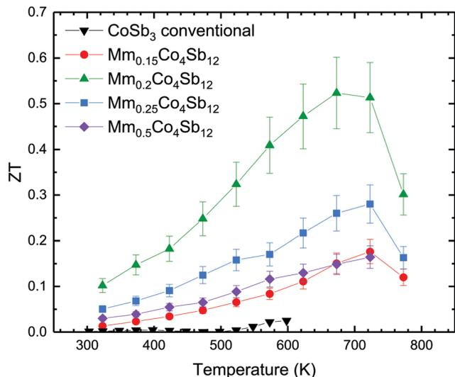
Fig. 7 Temperature dependence of the figure of merit of  $\text{MmCo}_4\text{Sb}_{12}$  and  $\text{CoSb}_3$ .  $\pm 15\%$  error bars are included in the graph, based on the accumulation of errors of 5% for the Seebeck coefficient, 5% for the thermal conductivity and 1.5% for the electrical resistivity.
