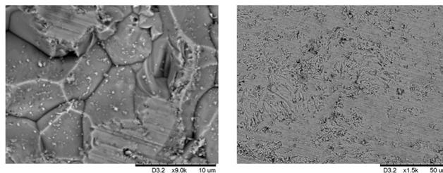
Fig. 3 SEM images of as-grown pellets of Mm<sub>0.2</sub>Co<sub>4</sub>Sb<sub>12</sub>. (a) ×9000 and (b) ×1500 magnification.
