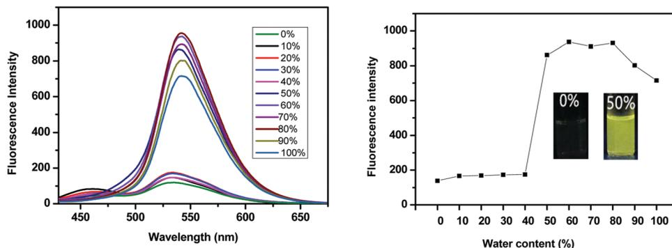
Fig. 3 Emission spectra of **SPF-2** in 1,4-dioxane and 1,4-dioxane/water mixtures with different water fractions (left). Plot of the emission intensity ( $I$ ) versus the composition of the aqueous mixtures of the **SPF-2** DMF solution (right). Solution concentration:  $10 \mu\text{M}$ ;  $\lambda_{\text{ex}}$ :  $400 \text{ nm}$ . Inset (right): photographs of **SPF-2** in pure 1,4-dioxane and 1,4-dioxane/water mixtures (50%) under  $365 \text{ nm}$  UV irradiation.
