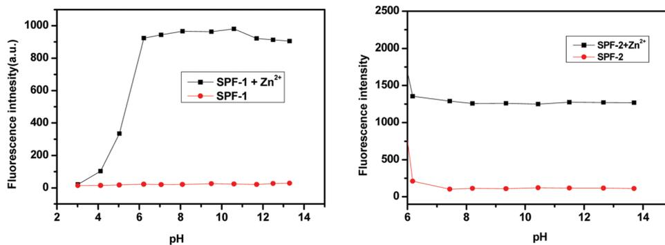
Fig. 12 Variation of fluorescence intensity at 488 nm for **SPF-1** solution with and without  $\text{Zn}^{2+}$  (1 equiv.) as a function of pH (left). Variation of fluorescence intensity at 535 nm for **SPF-2** solution with and without  $\text{Zn}^{2+}$  (1 equiv.) as a function of pH (right).
