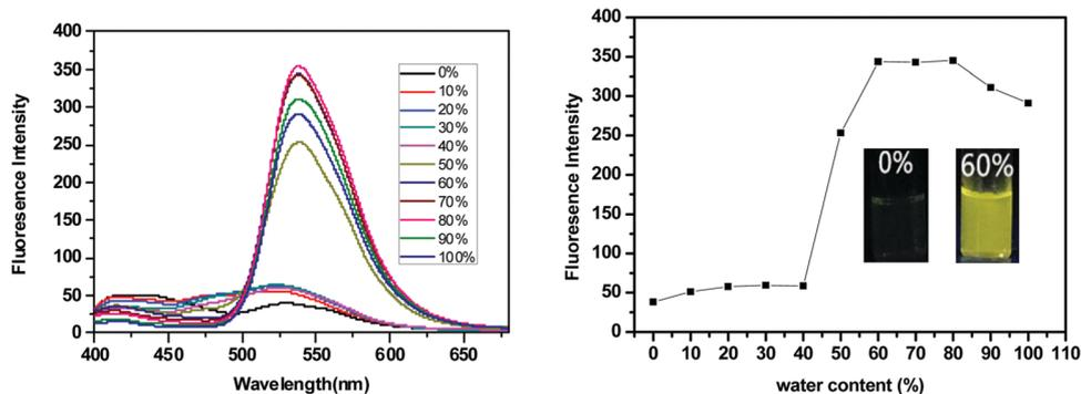
Fig. 2 Emission spectra of **SPF-1** in DMF and DMF/water mixtures with different water fractions (left). Plot of the emission intensity ( $I$ ) versus the composition of the aqueous mixtures of the **SPF-1** DMF solution (right). Solution concentration:  $10 \mu\text{M}$ ;  $\lambda_{\text{ex}}$ :  $362 \text{ nm}$ . Inset (right): photographs of **SPF-1** in pure DMF and DMF/water mixtures (60%) under  $365 \text{ nm}$  UV irradiation.
