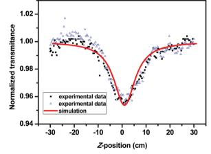
Fig. 13 Open Z-scan data of SPF-2 in THF.
