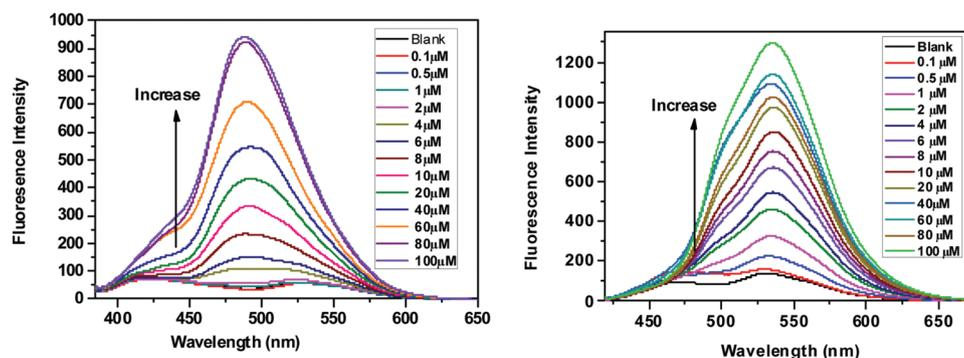
Fig. 5 Fluorescence spectra of **SPF-1** (10 μM) ( $\lambda_{\text{ex}} = 362$  nm) with varying concentrations of Zn<sup>2+</sup> in DMF/H<sub>2</sub>O (9 : 1, v/v) (left). Fluorescence spectra of **SPF-2** (10 μM) ( $\lambda_{\text{ex}} = 400$  nm) with varying concentrations of Zn<sup>2+</sup> in 1,4-dioxane/H<sub>2</sub>O (13 : 7, v/v) (right).
