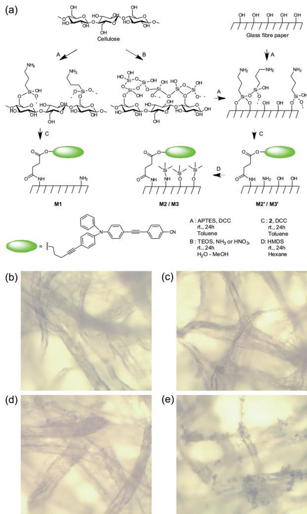
**Fig. 3** (a) Scheme representing the preparations of the different test strips **M1**, **M2'**, **M2**, **M3'**, and **M3**. Microscopy photographs of cellulose without coating (b) and silica-coated cellulose strip obtained (c) under acidic conditions (HNO<sub>3</sub>, #4), (d) with 0.7 equivalents of ammonia vs. TEOS (#6) and (e) 0.2 equivalents of ammonia vs. TEOS (#10).
