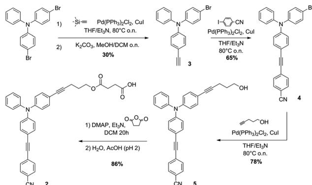
Scheme 2 Synthesis of the molecular probe **2**.
