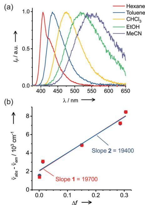
Fig. 1 (a) Normalized emission spectra of **2** in various solvents and (b) Lippert–Mataga correlations for CT dyes **1** and **2**. The error in the Stokes shift is 10 cm<sup>-1</sup> ( $C_1 = C_2 = 4 \mu\text{M}$ ,  $\lambda_{\text{exc}} = 340 \text{ nm}$ ).
