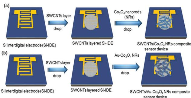
Fig. 2 Scheme illustrating the flow of the fabrication process (sensor devices) using (a)  $\text{Co}_3\text{O}_4$  NRs and (b) Au-decorated  $\text{Co}_3\text{O}_4$  NRs. The red spots on the NRs correspond to Au nanoparticles.
