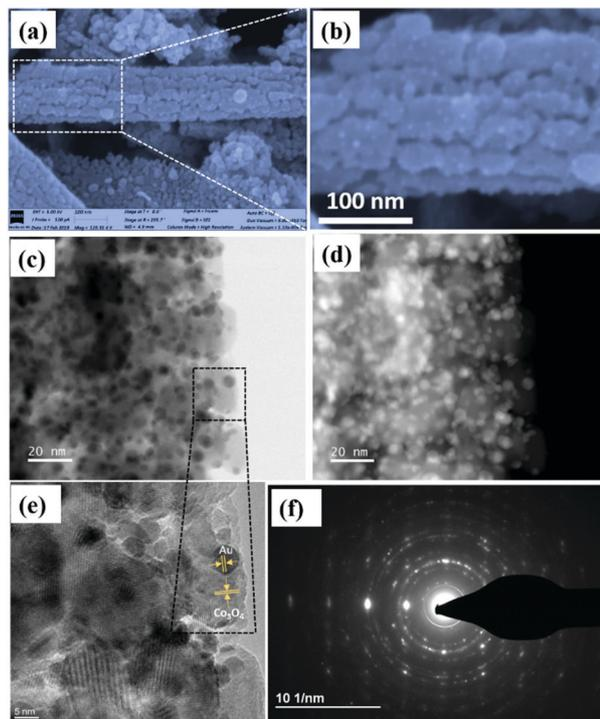
Fig. 5 (a and b) FESEM images, (c) TEM image, (d) HAADF image, (e) HR-TEM image recorded from the black dotted area of image (d), and (f) selected area diffraction (SAED) pattern of the 1-Au/Co<sub>3</sub>O<sub>4</sub> NR sample.
