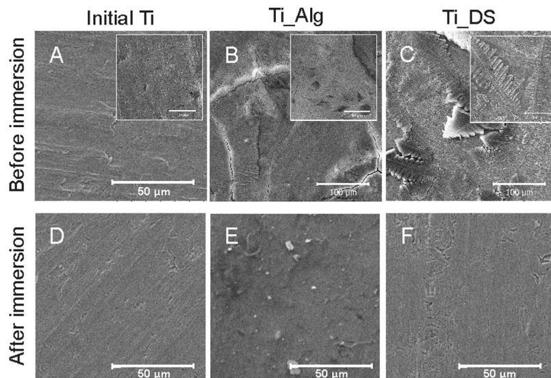
**Fig. 1** SEM images of the bare Ti surface before (A) and after the corrosion process (D); Ti plate coated with  $\text{Ca}^{2+}$ -crosslinked alginate hydrogel (Ti-Alg) before (B) and after the corrosion process (E); and Ti surface coated with dextran sulfate (Ti-DS) before (C) and after the electrochemical tests (F). The scale segment of the magnified image insets in the upper row is 10  $\mu\text{m}$ .
