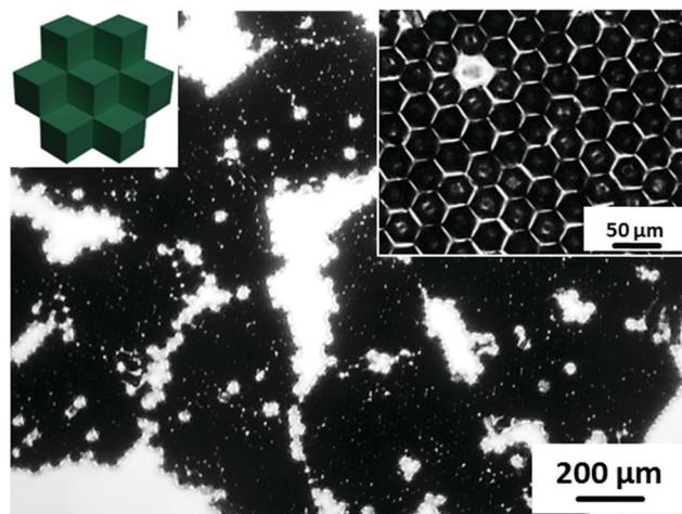
**Fig. 3** Optical microscopy image of close-packed hexagonal aggregates self-assembled from ODT/MUBiB functionalized cubes ( $\chi_{\text{ODT}} = 0.2$ ) at the water/air interface. The inset shows a higher magnification view of one aggregate.
