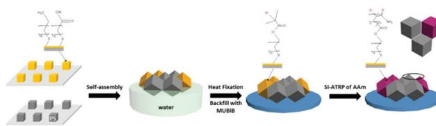
**Scheme 1** Fabrication of 3D microwells containing multiple differently functionalized surfaces (protein resistant: PAAm; protein attractive: PS) *via* self-assembly of different microcubes at the water/air interface.
