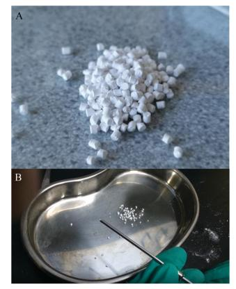
Fig. 3 (A) Optical image of granule A. (B) Granules were injected through a needle that is mainly used for bone cement.
