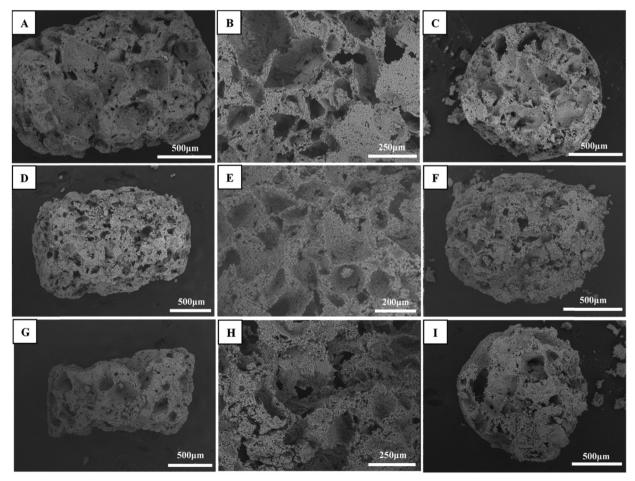
Fig. 4 Morphologies of granule A: (A) overview, (B) pore morphology, and (C) cross-section; granule B: (D) overview, (E) pore morphology, and (F) crosssection; and granule C: (G) overview, (H) pore morphology, and (I) cross-section.
