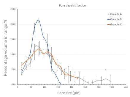
Fig. 6 Pore size distribution obtained from micro-CT (pore size below 5 μm was not counted): granule A, granule B, and granule C. The profile shows the percentage of the volume in a specific pore-size range (x axis) in the total volume of the full pore-size range.
