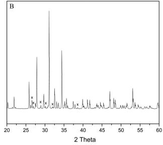
Fig. 1 (A) XRD patterns of granules after moulding (bottom), after leaching (middle) and after leaching and autoclaving (top). Peaks from  $\alpha$ -TCP, HA and PEG are marked. (B) XRD pattern of  $\beta$ -TCP, x:  $\beta$ -calcium pyrophosphate.
