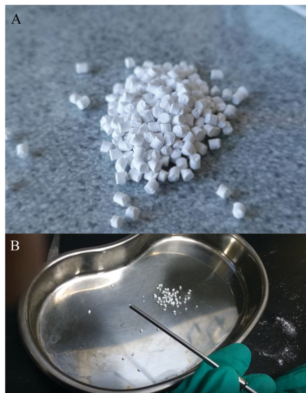
Fig. 3 (A) Optical image of granule A. (B) Granules were injected through a needle that is mainly used for bone cement.
