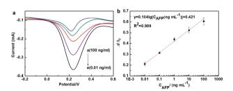
Fig. 5 (a) Differential pulse voltammetry of the as-prepared immunosensors in the presence of AFP with different concentrations (0.01 ng ml<sup>-1</sup>,  $0.1 \text{ ng ml}^{-1}$ ,  $1 \text{ ng ml}^{-1}$ ,  $10 \text{ ng ml}^{-1}$ , and  $100 \text{ ng ml}^{-1}$ ). (b) Corresponding calibration curve for AFP detection, the error bars represent the standard deviation obtained from three measurements (n = 3).
