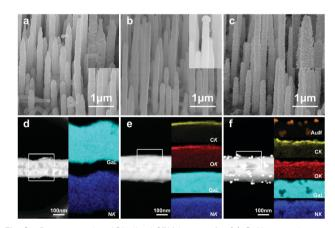
Fig. 2 Representative 40°-tilted SEM images for (a) GaN nanowire array, (b) GaN nanowire array/PDA and (c) GaN nanowire array/PDA/Au NPs; insets display the morphology of individual nanowires after each assembly step. STEM images for an individual nanowire after each step and its corresponding spatially resolved elemental mapping are shown in (d-f), respectively. The selected areas for compositional analysis are marked by white squares at the left side
