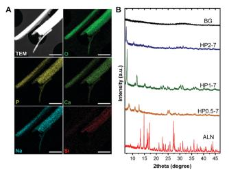
Fig. 3 (A) Scanning TEM image and EDX elemental maps of single HP1-7 particles. (B) Powder XRD spectra of different particle types. Scale bars in images correspond to 1 µm.
