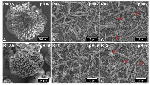
Fig. 1 Scanning electron micrographs of hybrid particles precipitated at different Ca<sub>BG</sub>/ALN ratios (R) and pH values after 3 days of incubation at 37 °C. Red arrows indicate bioactive glass residues.
