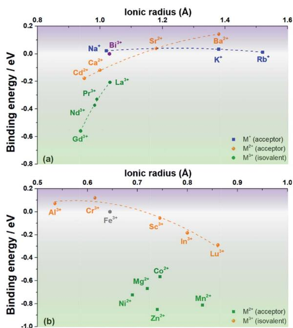
Fig. 2 Binding energies of a cation substituent-oxygen vacancy associate as a function of ionic radius for cations that prefer (a) the Bi site and (b) the Fe site of rhombohedral BiFeO<sub>3</sub>.
