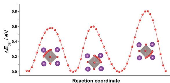
Fig. 1 Three distinct energy profiles for oxide-ion migration in pure, rhombohedral BiFeO<sub>3</sub>. Key: Bi (purple); Fe (silver); O (red). The traced trajectories reveal that the migrating ion follows a curved pathway through a triangular aperture defined by two A-site cations and one B-site cation, bowing away from the edge of the BO<sub>6</sub> octahedron, as observed previously.<sup>17</sup>
