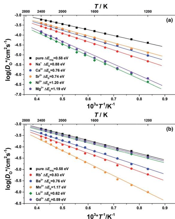
Fig. 3 Oxygen tracer diffusion coefficients ( $D_{\text{O}}^*$ ) for various substituted, rhombohedral BiFeO<sub>3</sub> compositions obtained from MD simulations against inverse temperature: (a) data for substituent cations that should maximise  $D_{\text{O}}^*$ ; (b) data for substituent cations that should minimise  $D_{\text{O}}^*$ .
