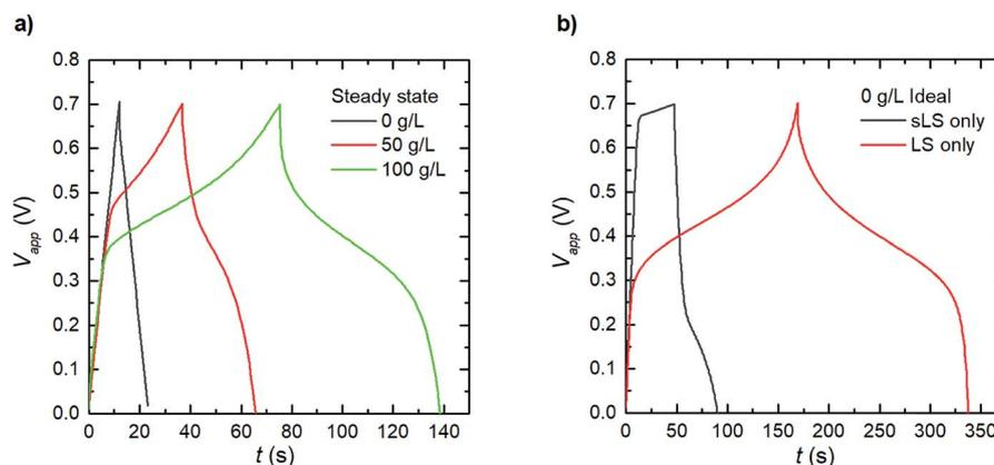
Fig. 5 Simulated electrode response under galvanostatic charge–discharge at  $1689 \mu\text{A}$  ( $2 \text{ A g}^{-1}$ ) for 1\_2 electrodes. (a) At steady operation (after long cycling), and (b) for idealized cases where LS is confined in electrode domain in only solid (sLS) or dissolved (LS) form.
