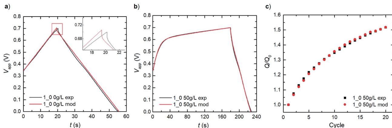
Fig. 3 Comparison of model and experimental results for galvanostatic charge–discharge at 566  $\mu\text{A}$  ( $2 \text{ A g}^{-1}$ ): (a) PEDOT:PSS + NFC without preloaded LS (1\_0) and 0 g L<sup>-1</sup> LS in electrolyte (no changes with cycling). (b) Cycle 1 of 1\_0 electrode with initial 50 g L<sup>-1</sup> LS dissolved in bulk electrolyte. (c) Relative discharge capacity recorded for 20 cycles following (b).  $L_E$  is 52  $\mu\text{m}$  in both (a) and (b).
