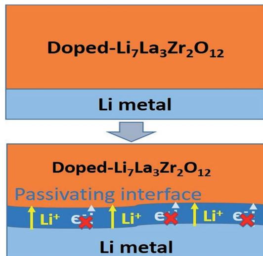
Fig. 7 Improvement of Li|LLZOM (M = dopants) interfacial stability via the formation of a passivating interface layer.
