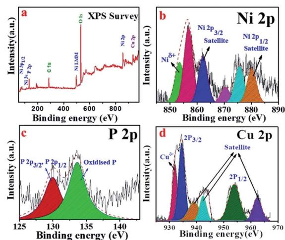
**Fig. 4** (a) XPS survey spectra of Cuf@Ni<sub>5</sub>P<sub>4</sub>, and high-resolution deconvoluted XPS spectra for: (b) Ni 2p; (c) P 2p; and (d) Cu 2p.
