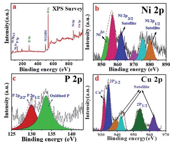
**Fig. 4** (a) XPS survey spectra of Cuf@Ni<sub>5</sub>P<sub>4</sub>, and high-resolution deconvoluted XPS spectra for: (b) Ni 2p; (c) P 2p; and (d) Cu 2p.
