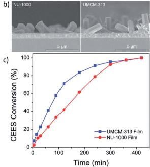
Fig. 13 (a) General structure of three MOFs, PCN-222/MOF-545, NU-1000, and UMCM-313, used as a thin-film protective coating against mustard gas simulant. (b) NU-1000 and UMCM-313 thin films prepared using layer-by-layer techniques on FTO substrates and (c) their reaction profiles for the photocatalytic oxidation of CEES. Adapted with permission.<sup>226</sup> Copyright 2018 American Chemical Society.
