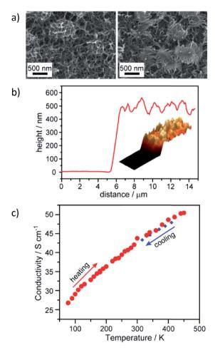
Fig. 10 a) SEM micrographs of  $Ni_3$ (HITP)<sub>2</sub> films with 500 nm thickness measured via (b) AFM. (c) van der Pauw conductivity measurements at various temperatures show reversible increase in conductivity for 500 nm thick films on quartz. Adapted with permission. Copyright 2014 American Chemical Society.
