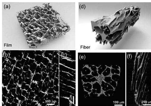
Fig. 3 The 3D reconstructed structure from the SR- $\mu$ CT data of (a) the LLZO film and (d) longitudinal section. The cross-sections for the film are shown in (b) top and (c) left views. (e) and (f) are the top and left views of the LLZO longitudinal section.
