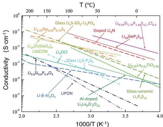
Fig. 7 Thermal evolution of ionic conductivity for different types of solid electrolytes. Reprinted with permission.<sup>81</sup> Copyright© 2018, Royal Society of Chemistry.
