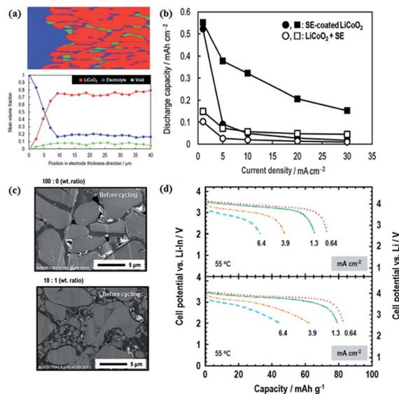
**Fig. 12** (a) Volume fractions of respective materials along the electrode thickness; (b) electrochemical performance of S-SE-coated LiCoO<sub>2</sub> and LiCoO<sub>2</sub> + S-SE; (c) S-SE-coated LiCoO<sub>2</sub> particles with different grain sizes; (d) electrochemical performances of different cathode compositions. Reproduced with permission.<sup>109</sup> Copyright© 2017, Royal Society of Chemistry.
