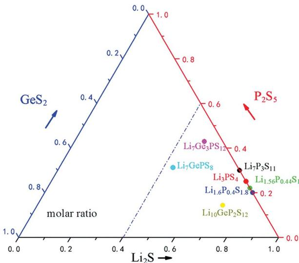
Fig. 5  $\text{Li}_2\text{S}$ - $\text{P}_2\text{S}_5$ - $\text{GeS}_2$  ternary phase diagrams.
