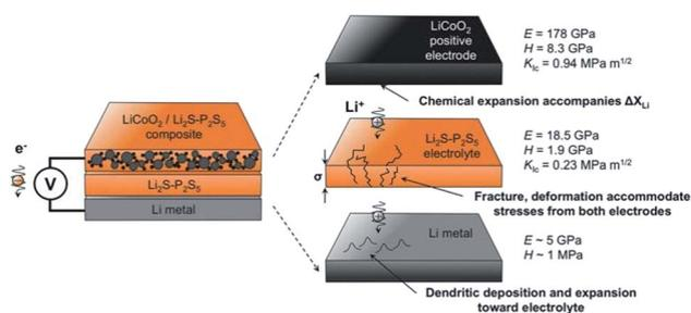
Fig. 20 Summary of mechanical performance data for  $\text{Li}_2\text{S-P}_2\text{S}_5$  (LPS) in the context of all-solid-state batteries. Reprinted with permission.<sup>166</sup> Copyright© 2017, John Wiley and Sons.
