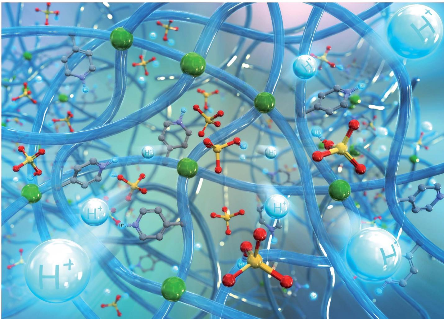
Showcasing a study on proton-conductive polymer membranes exhibiting anhydrous conductivity higher than  $100 \text{ mS cm}^{-1}$  at around  $100 \text{ }^\circ\text{C}$ , by Prof. Atsushi Noro at Nagoya University and Dr Naoki Nakamura at Toyota Motor Corporation.
