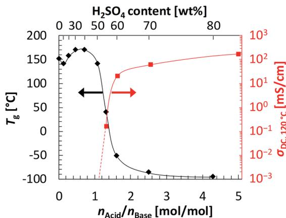
Fig. 4  $T_g$  of P/H<sub>2</sub>SO<sub>4</sub> mixtures (left axis) and anhydrous conductivity at 120 °C of CL-P/H<sub>2</sub>SO<sub>4</sub> membranes (right axis) against H<sub>2</sub>SO<sub>4</sub>/pyridyl group molar ratio ( $n_{\text{Acid}}/n_{\text{Base}}$ ) and the content of H<sub>2</sub>SO<sub>4</sub> in mixtures. Solid and broken lines are drawn as guide for eyes.
