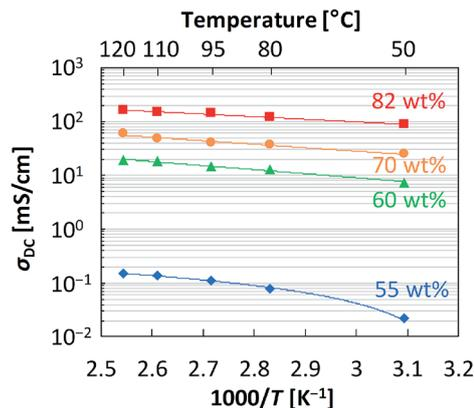
Fig. 3 Anhydrous conductivity versus reciprocal absolute temperature for several CL-P/H<sub>2</sub>SO<sub>4</sub> membranes. Solid lines are drawn as guide for eyes.
