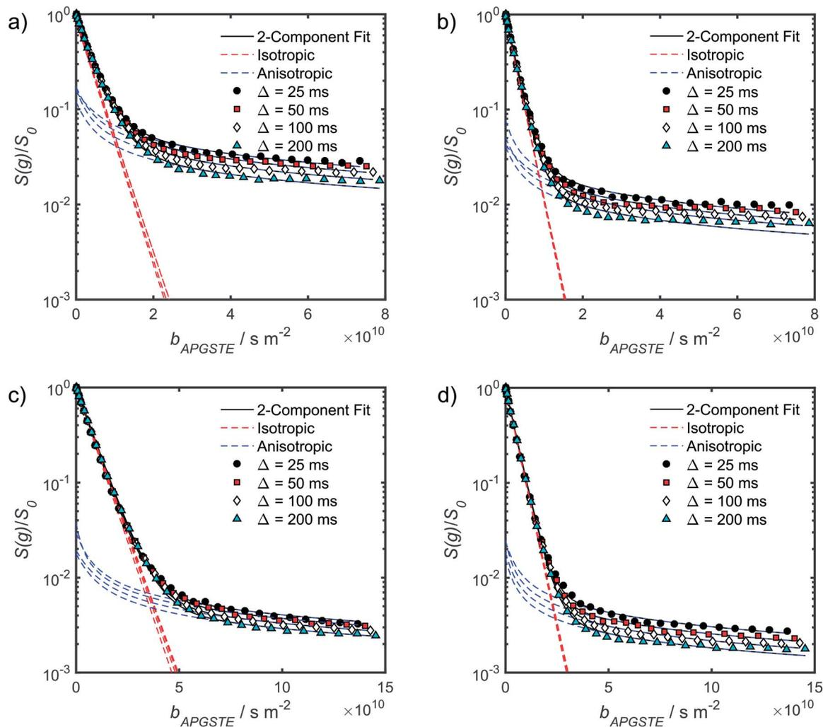
Fig. 5 APGSTE data for  $\text{PrSO}_3\text{H/MM-SBA-15}$  catalysts: PFG NMR signal attenuation curves for (a and b) cyclohexane saturated and (c and d) dodecane-saturated  $\text{PrSO}_3\text{H/MM-SBA-15}$  catalysts with respective 150 nm and 430 nm macropores. Two-component fits to the acquired data points utilised eqn (6); isotropic and anisotropic fitted components are shown in red and blue respectively.
