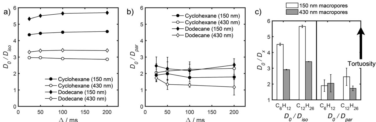
Fig. 7 (a and b) Effective tortuosity parameters as a function of observation time, and (c) comparative summary for  $\text{PrSO}_3\text{H/MM-SBA-15}$  with different macropores and probe molecules ( $\Delta = 100$  ms for  $D_0/D_{iso}$  values and  $\Delta = 25$  ms for  $D_0/D_{par}$  values).
