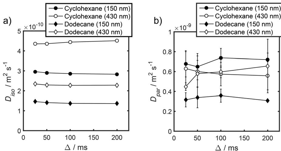
Fig. 6 (a)  $D_{iso}$  and (b)  $D_{par}$  values obtained by fitting APGSTE data to eqn (6). Macropore diameters are indicated in parentheses. Errors represent  $\pm 1$  standard deviation of three measurements of three different samples and are too small to be observed in (a).
