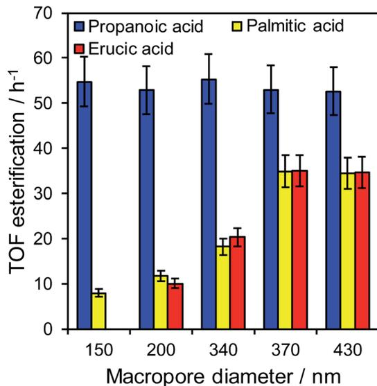
Fig. 3 Turnover frequencies for propanoic acid, palmitic acid, and erucic acid esterification over PrSO<sub>3</sub>H/MM-SBA-15 as a function of macropore diameter.
