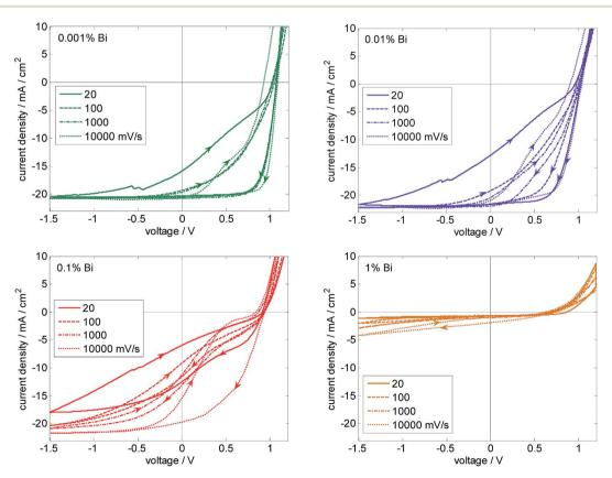
Fig. 3 JV hysteresis loops starting from 1.2 V for various voltage sweep rates measured at solar cells with different Bi concentrations. Reduced  $J_{SC}$  and FF upon addition of Bi are mainly due to a strong dependence of charge extraction on the electric field. (The 0% Bi device behaves similarly as the 0.001%, see Fig. S2†).
