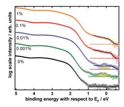
Fig. 7 UPS measurements of  $Cs_{0.1}FA_{0.9}Pb(Br_{0.1}I_{0.9})_3$  films with different Bi concentration (on FTO) showing the valence band region in a semi-logarithmic plot. For intermediate Bi concentrations, a deep defect state (yellow) is observable which is superimposed by a broader density of states extending to the Fermi edge (black) for higher concentrations.
