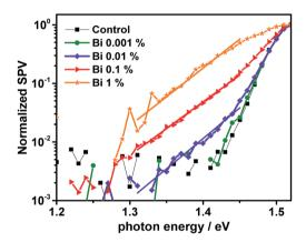
Fig. 6 Surface photovoltage (SPV) measurements on samples with  $Cs_{0.1}FA_{0.9}Pb(Br_{0.1}I_{0.9})_3$  showing the presence of tail states with higher Bi content. The lines indicate an exponential fit between 1.3 and 1.45 eV, yielding characteristic energies of 47, 47, and 46 meV, for [Bi] = 1, 0.1, and 0.01%, respectively.
