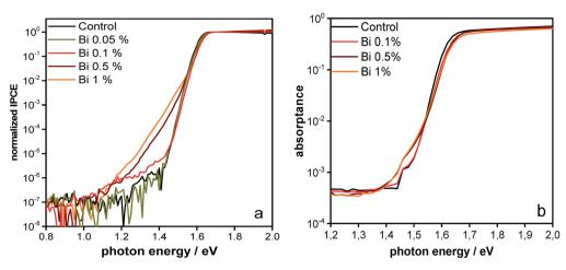
Fig. 5 Sensitive optical measurements at the band edge (a) IPCE measured by FTPS and (b) PDS. Both measurements show that larger amounts of Bi introduce optically detectable tail states.
