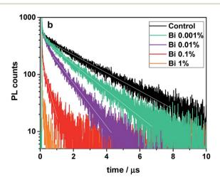
Fig. 4 Photoluminescence of perovskite films (a) absolute PL spectra showing that adding Bi reduces the PL yield so substantially that it is hardly detectable for [Bi] = 1%. (b) Transient PL with a reduced decay time for higher Bi concentrations. The white lines are mono-exponential fits and span the time range selected for the fits.
