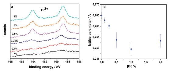
Fig. 8 Structural characterization of perovskite films containing Bi (a) XPS spectra showing the characteristic signal for Bi<sup>3+</sup> which increases for higher Bi content. (b) Lattice parameter deduced from fitting XRD spectra. Incorporation of Bi decreases the lattice parameter.
