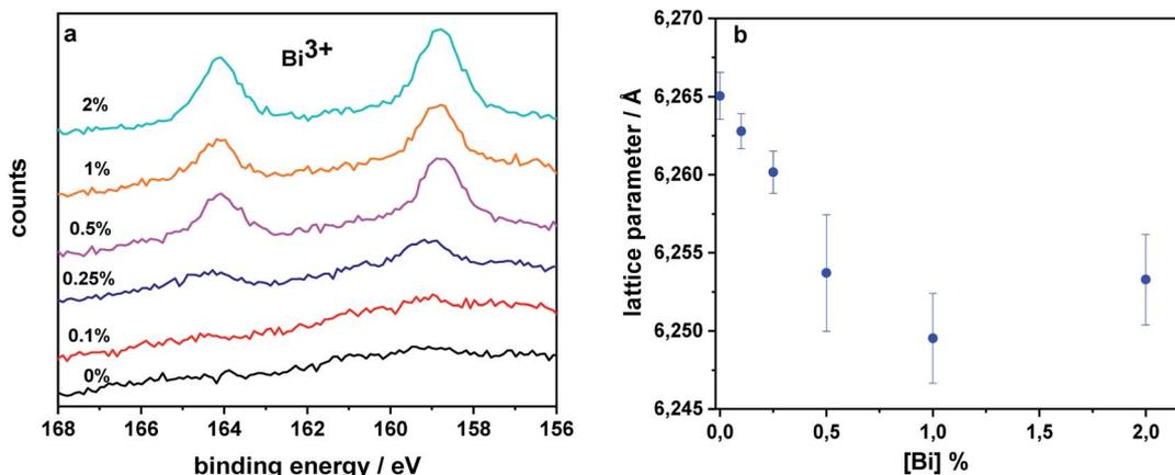
Fig. 8 Structural characterization of perovskite films containing Bi (a) XPS spectra showing the characteristic signal for Bi<sup>3+</sup> which increases for higher Bi content. (b) Lattice parameter deduced from fitting XRD spectra. Incorporation of Bi decreases the lattice parameter.
