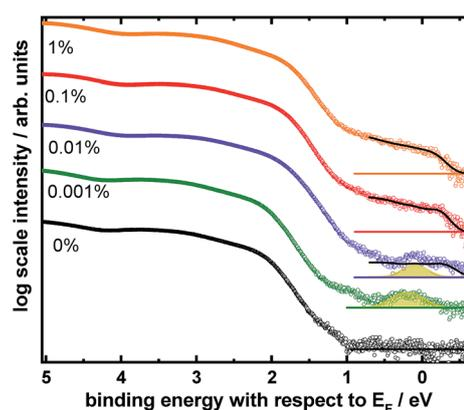
Fig. 7 UPS measurements of  $\text{Cs}_{0.1}\text{FA}_{0.9}\text{Pb}(\text{Br}_{0.1}\text{I}_{0.9})_3$  films with different Bi concentration (on FTO) showing the valence band region in a semi-logarithmic plot. For intermediate Bi concentrations, a deep defect state (yellow) is observable which is superimposed by a broader density of states extending to the Fermi edge (black) for higher concentrations.
