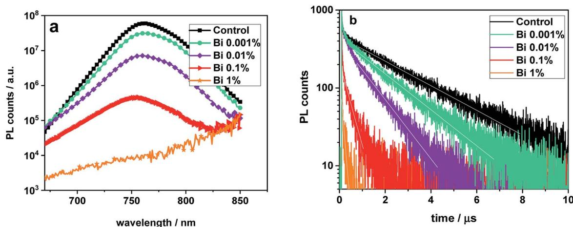
**Fig. 4** Photoluminescence of perovskite films (a) absolute PL spectra showing that adding Bi reduces the PL yield so substantially that it is hardly detectable for  $[Bi] = 1\%$ . (b) Transient PL with a reduced decay time for higher Bi concentrations. The white lines are mono-exponential fits and span the time range selected for the fits.
