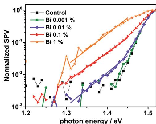
Fig. 6 Surface photovoltage (SPV) measurements on samples with  $\text{Cs}_{0.1}\text{FA}_{0.9}\text{Pb}(\text{Br}_{0.1}\text{I}_{0.9})_3$  showing the presence of tail states with higher Bi content. The lines indicate an exponential fit between 1.3 and 1.45 eV, yielding characteristic energies of 47, 47, and 46 meV, for [Bi] = 1, 0.1, and 0.01%, respectively.
