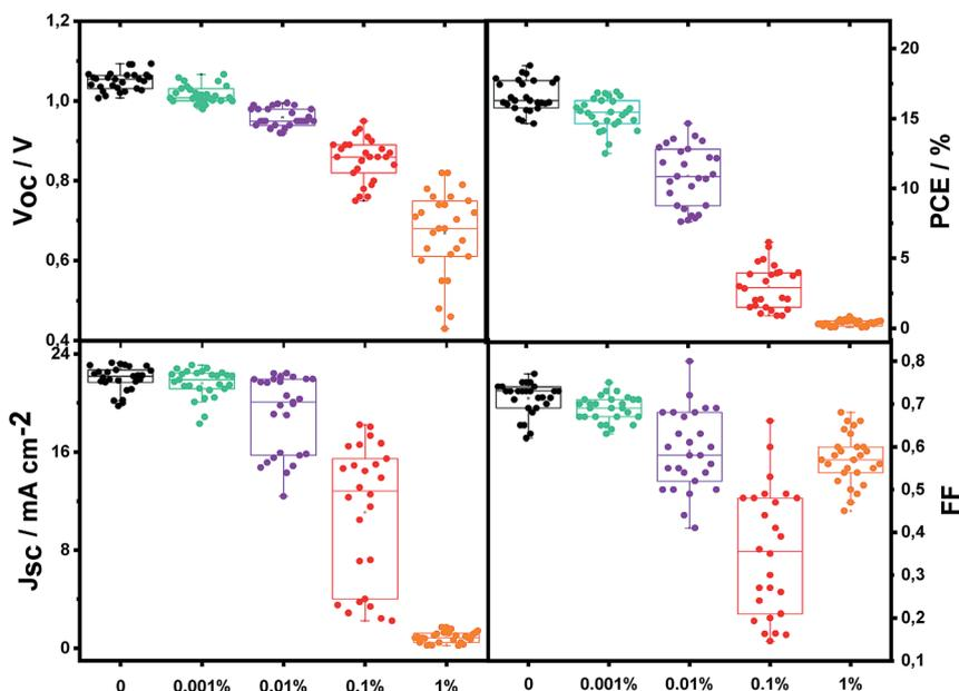
Fig. 1 Characteristic parameters for solar cells containing different concentrations of intentionally added Bi denoted in at% referred to Pb. Even a concentration of 10 ppm results in a decrease of performance.
