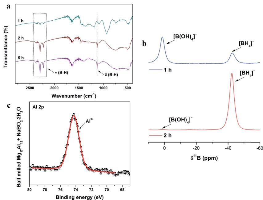
Fig. 3 (a) FTIR spectra of the 1, 2 and 5 h ball milled products of Mg<sub>17</sub>Al<sub>12</sub> and NaB(OH)<sub>4</sub> mixtures (in a molar ratio of 4 : 35). (b) <sup>11</sup>B NMR spectra of the 1 and 2 h ball milled products of Mg<sub>17</sub>Al<sub>12</sub> and NaB(OH)<sub>4</sub> mixtures (in a 4 : 35 molar ratio). (c) XPS spectra of Al 2p of the 1 h ball milled products of Mg<sub>17</sub>Al<sub>12</sub> and NaB(OH)<sub>4</sub> mixtures (in a 4 : 35 molar ratio).
