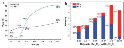
Fig. 2 (a) Yields of the ball milled products of  $Mg_{17}Al_{12}$  and  $NaB(OH)_4$  mixtures (in 4 : 35 and 4 : 17 molar ratios) for different milling times. (b) Yields of the 10 and 20 h ball milled products of  $Mg_{17}Al_{12}$  and  $NaB(OH)_4$  mixtures with different mole ratios.
