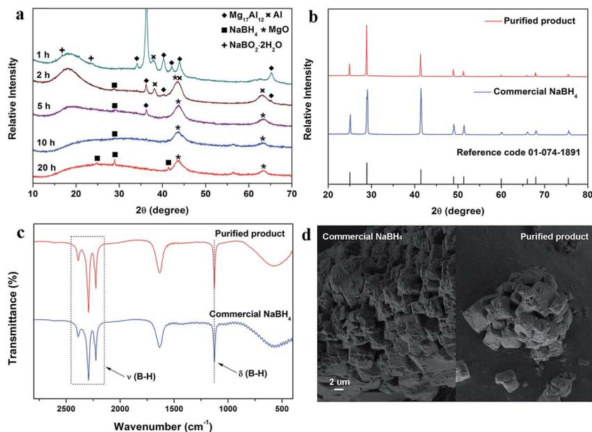
Fig. 1 (a) XRD patterns of the 5, 7.5, 10 and 20 h ball milled products of Mg<sub>17</sub>Al<sub>12</sub> and NaB(OH)<sub>4</sub> mixtures (in a 4 : 35 molar ratio). (b) XRD patterns of the purified product (red line) and commercial NaBH<sub>4</sub> (blue line). (c) FTIR spectra of the purified product (red line) and the commercial NaBH<sub>4</sub> (blue line). (d) SEM images of the commercial NaBH<sub>4</sub> (left) and the purified product (right).
