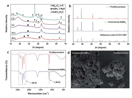
Fig. 1 (a) XRD patterns of the 5, 7.5, 10 and 20 h ball milled products of  $Mg_{17}Al_{12}$  and  $NaB(OH)_4$  mixtures (in a 4 : 35 molar ratio). (b) XRD patterns of the purified product (red line) and commercial  $NaBH_4$  (blue line). (c) FTIR spectra of the purified product (red line) and the commercial  $NaBH_4$  (blue line). (d) SEM images of the commercial  $NaBH_4$  (left) and the purified product (right).
