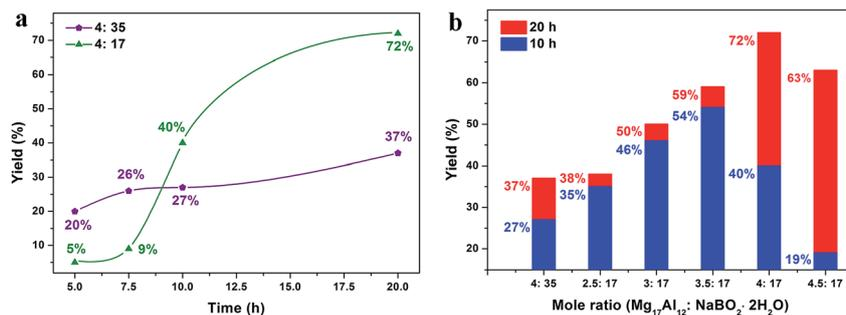
Fig. 2 (a) Yields of the ball milled products of Mg<sub>17</sub>Al<sub>12</sub> and NaB(OH)<sub>4</sub> mixtures (in 4 : 35 and 4 : 17 molar ratios) for different milling times. (b) Yields of the 10 and 20 h ball milled products of Mg<sub>17</sub>Al<sub>12</sub> and NaB(OH)<sub>4</sub> mixtures with different mole ratios.
