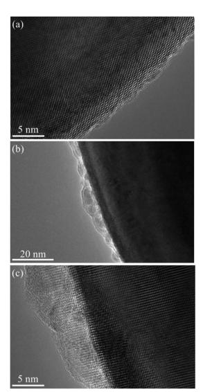
Fig. 7 HRTEM images of STO powder before and after the performance test: (a) raw powder and (b) and (c) STO powder scraped from the cell after electrochemical performance testing.
