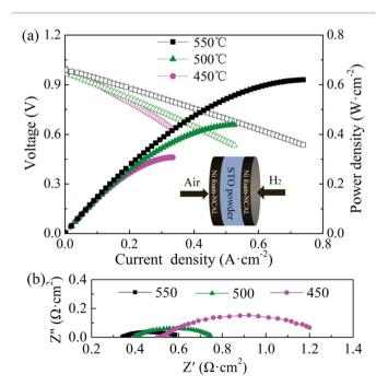
Fig. 2 (a) IV–IP curves and (b) impedance spectra of the cell (under open circuit) at 450, 500, and 550  $^{\circ}\text{C}.$
