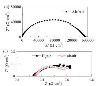
Fig. 4 Impedance spectra of the cell operated at 550 °C in different atmospheres: (a) with air on both the sides before the performance test in H<sub>2</sub> and (b) with H<sub>2</sub>/air and air/air sequentially (each pair of gases was flown for 1 h for the EIS test).
