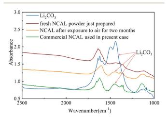
Fig. 10 FTIR spectra of  $\rm Li_2CO_3$  and NCAL powders treated under different conditions.
