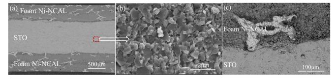
Fig. 3 (a) Cross-sectional SEM images of the cell, (b) magnified image of the electrolyte, and (c) magnified image of the interface of the Ni foam-NCAL electrode and the STO electrolyte.
