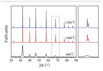
Fig. 1 XRD patterns of the STO powder after sintering at 800, 1000, and 1200 °C in air for 5 h.
