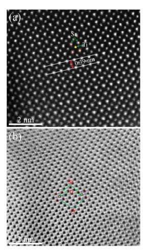
**Fig. 6** HRTEM images of STO powder before the performance test. (a) HAADF-STEM image and (b) ABF-STEM image.
