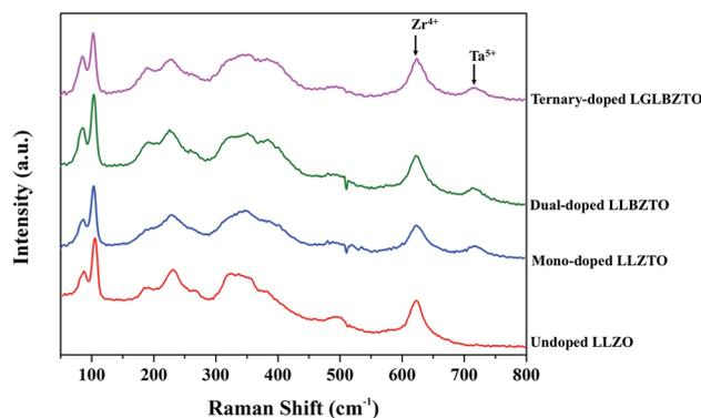
**Fig. 2** Raman spectra of the undoped LLZO, mono-doped LLZTO, dual-doped LLBZTO, and ternary-doped LGLBZTO in the range of 50–800 cm<sup>-1</sup>.
