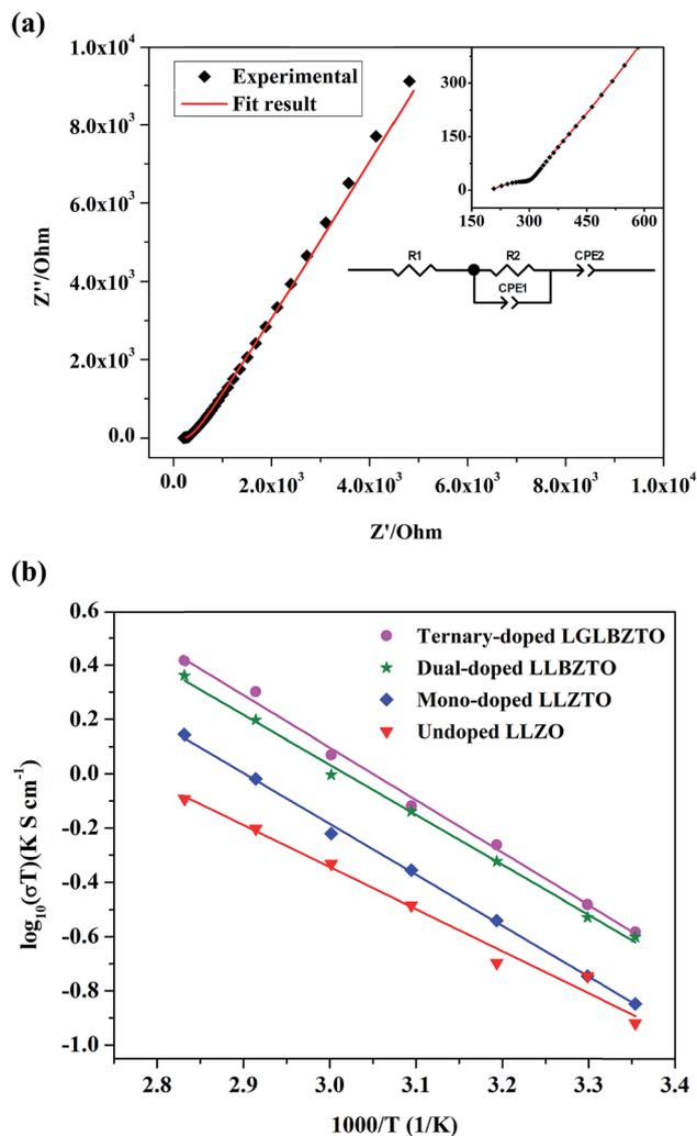
Fig. 4 (a) AC impedance plot of the garnet-type ternary-doped LGLBZTO  $\text{Li}_{6.65}\text{Ga}_{0.05}\text{La}_{2.95}\text{Ba}_{0.05}\text{Zr}_{1.75}\text{Ta}_{0.25}\text{O}_{12}$ . The inset shows partially enlarged graph at the high frequency region. The equivalent circuit is used to fit the curve. (b) Arrhenius plot of the undoped LLZO, mono-doped LLZTO, dual-doped LLBZTO, and ternary-doped LGLBZTO.
