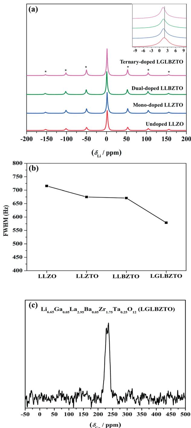
Fig. 6 (a)  $^7\text{Li}$  MAS NMR and (b) FWHM of the central transition line width for the undoped LLZO, mono-doped LLZTO, dual-doped LLBZTO, and ternary-doped LGLBZTO. The inset shows the magnified scale (\* spinning sidebands). (c)  $^{71}\text{Ga}$  NMR spectrum for the ternary-doped LGLBZTO showing a single broad signal at 210–255 ppm. The weak signals correspond to the spinning sidebands.
